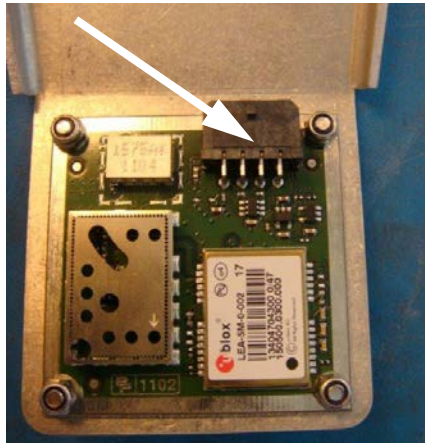
Figure 8-30: Connector for GPS PCB
