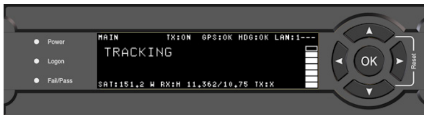
Figure 4-2: ACU: LEDs, display and keypad (detailed)
