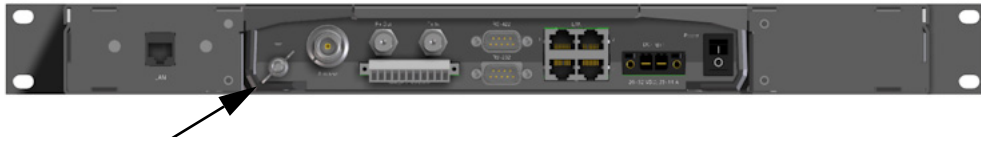
Figure 3-35: ACU, 19" rack version, ground stud
