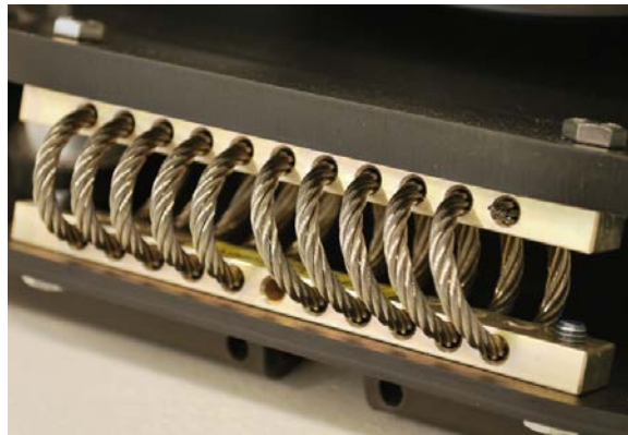
Figure 8-119: Wire-rope isolator in good condition
