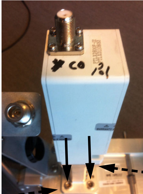
Figure 8-106: LNB, removing (SAILOR 800/900 VSAT variant A)
