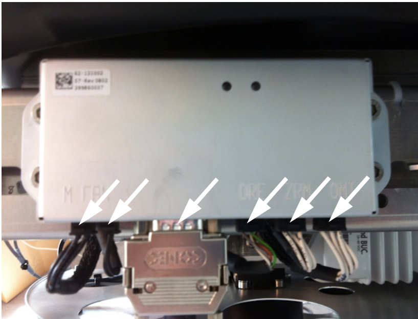
Figure 8-41: Polarisation Motor Module, remove connectors
