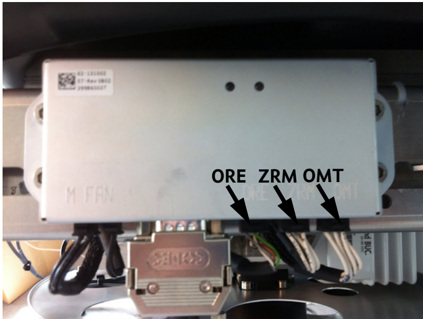
Figure 8-43: Polarisation Motor Module, inserting
