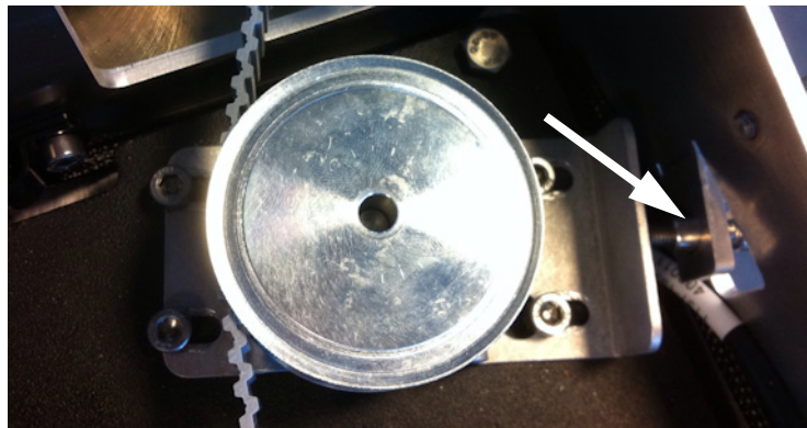
Figure 8-61: Azimuth encoder, adjust belt tension
