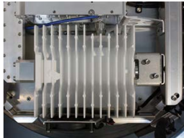
Figure 8-102: Block Up Converter (BUC) (SAILOR 800 picture)
