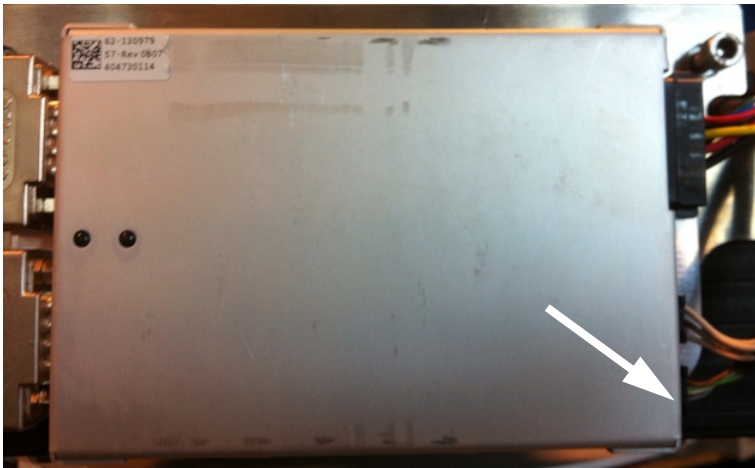
Figure 8-59: Azimuth DDM, disconnect connector
