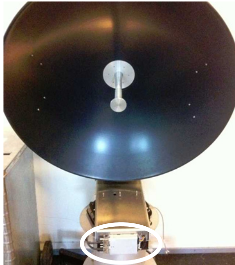
Figure 8-39: location of the Azimuth DDM (SAILOR 900 picture)
