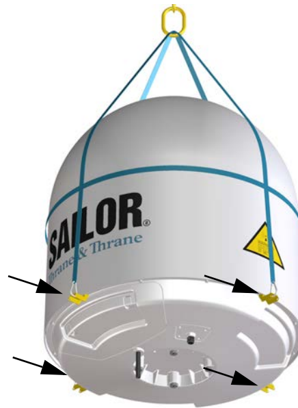
Figure 3-22: SAILOR 900: ADU installation, webbed sling attached to the 4 lifting brackets
