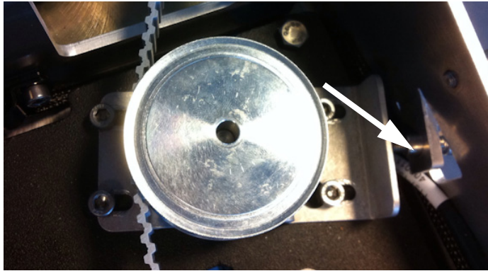
Figure 8-79: Azimuth drive belt, adjust belt tension
