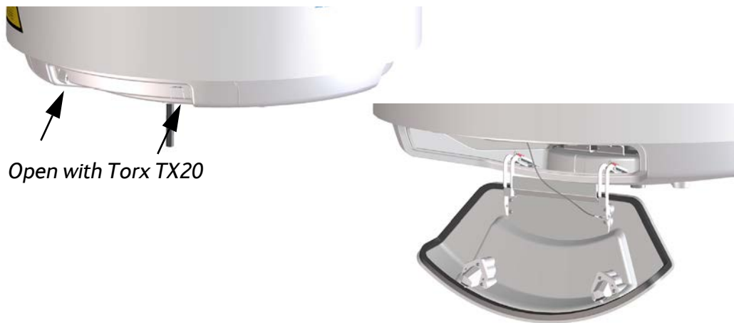
Figure 3-28: SAILOR 900: Opening the service hatch
