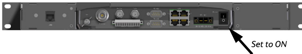
Figure 3-33: ACU, On/off switch at the back
