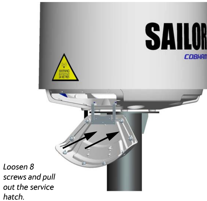
Figure 3-30: SAILOR 800: Removing the service hatch
