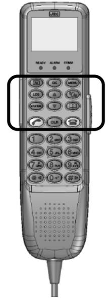
**Fig. 3.4.2 Functional button section**
