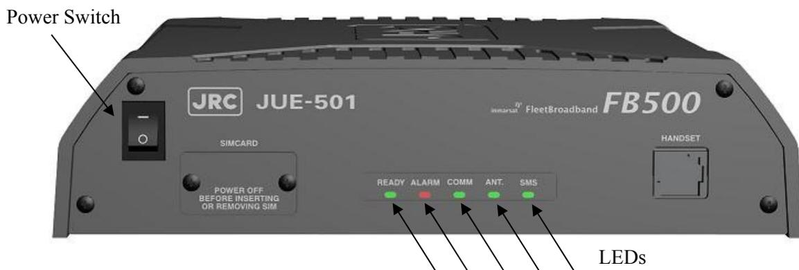
Fig.4.1.3a Power switch and LEDs of Main unit
