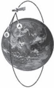
The location of the distress signal is determined by taking measurements of the doppler shift of the EPIRB frequency when the satellite first approach and then pass the EPIRB.
