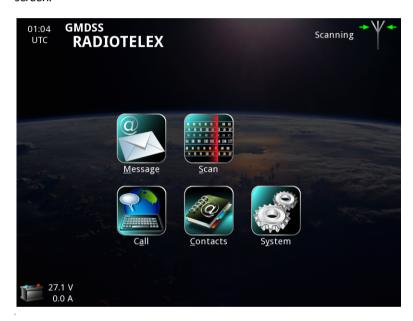
The Radiotelex application starts up automatically when the Message Terminal is powered. Note that the Message Terminal must always be powered in a GMDSS system.
