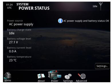
2. To see the power settings, select **Settings**... in the lower right corner of the **POWER STATUS** page. The battery settings are displayed.
