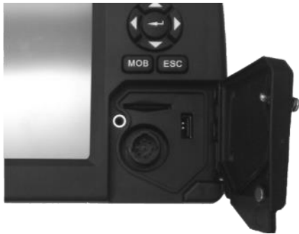
Figure 61- CDU Front ports
