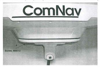
Please note that the pole mounting option does not meet IEC 60945, section 8.7 ("ability to withstand vibration").
