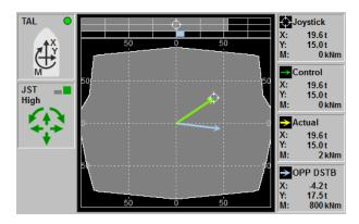
Figure 10.8: Thrust ability diagram. AWC function is OFF
