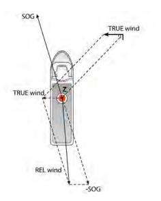
Figure D.1: True and relative (apparent) wind
