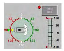
Figure 6.46: A power limited thruster indication example
