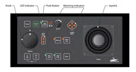
Figure 2.24: Control Panel Controls, Buttons and Indicators (MCP and PCP)
