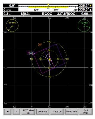
Figure 10.102: Map Window, "Foot Print" softkey is enabled
