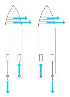
Figure 6.29: Thrust Allocation Modes: Starboard Ahead and Port Ahead
