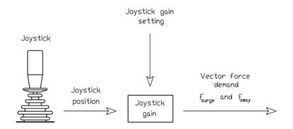
Figure 2.34: Joystick gain diagram
