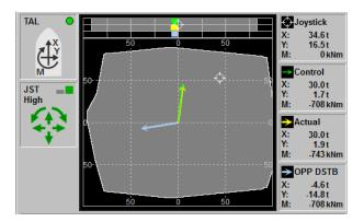
Figure 10.9: Thrust ability diagram. AWC function is ON
