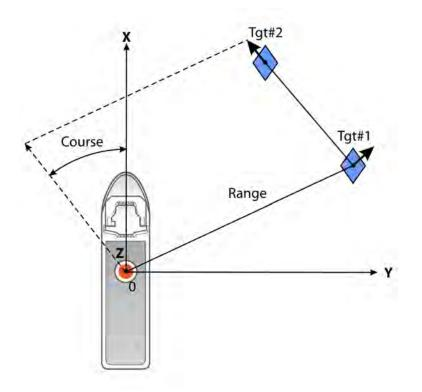
Figure 10.25: Multi-Target Following Mode: Coordinate Systems
