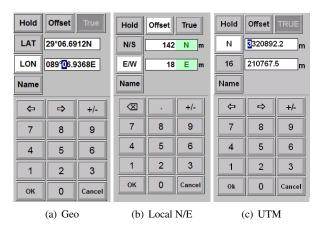
Figure 8.3: The waypoint set up dialogue for the different coordinate systems
