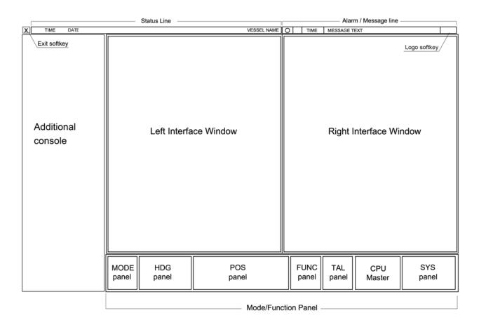
Figure 5.3: The Wide Screen Layout with Additional Left Console
