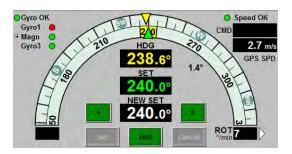
Figure 10.51: The Autopilot Heading Indicator
