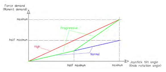
Figure 2.35: Joystick limits and gain types
