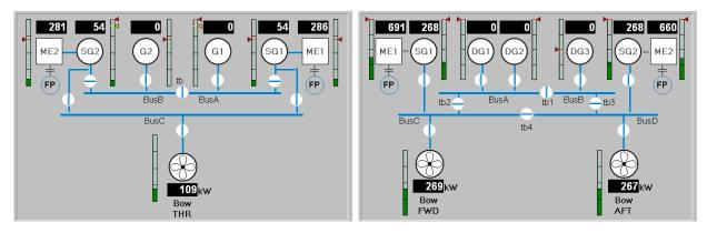
Figure 6.37: Power Mimic Diagram Examples
