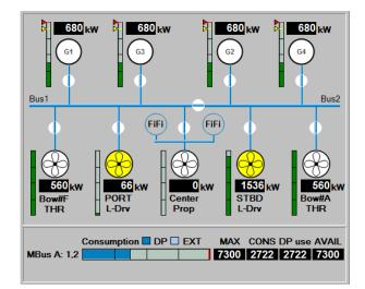
Figure 6.47: An example of power limites thrusters in the Power mimic diagram
