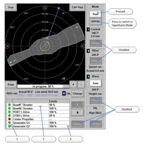
Figure 10.61: The Capability View in Real Mode
