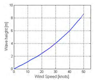
Figure 10.62: Relationship between Wave Height and Wind Speed
