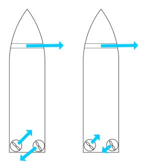
Figure 6.30: Thrust Allocation Modes: High and Low Bias
