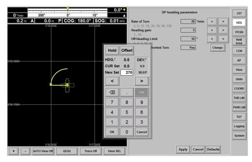
Figure 5.23: The turn track in case Always Use Shortest Turn=Yes
