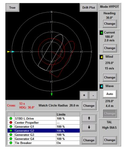
Figure 10.74: Drift Plot Window
