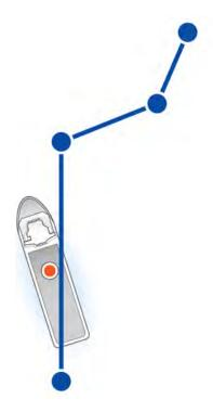
Figure 9.13: Position mode: LS Track Control
