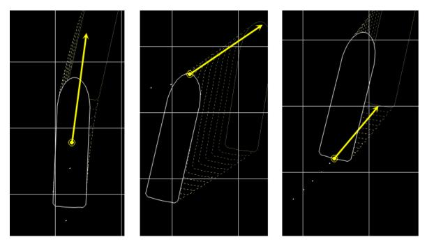
Figure 10.3: COR position: COR at Center, Bow, Stern
