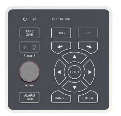
Figure 2.17: Control Panel Controls, Buttons and Indicators (MCP and PCP)
