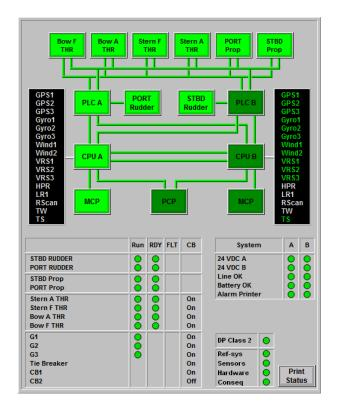
Figure 10.93: System Monitor Window Example — DP Class 2 System
