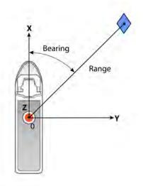
Figure 10.18: Single Target Following Mode: Coordinate Systems
