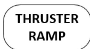
The main task of the Ramp Block is to change the actual Set Point to the new Set Point by increasing or decreasing as fast as the thruster is able to follow. Second task of the Ramp Block is to check whether the feedback signal matches the Set Point. The Ramp Block also calculates the force after ramp. This is the force that is actually delivered by the thrusters.
