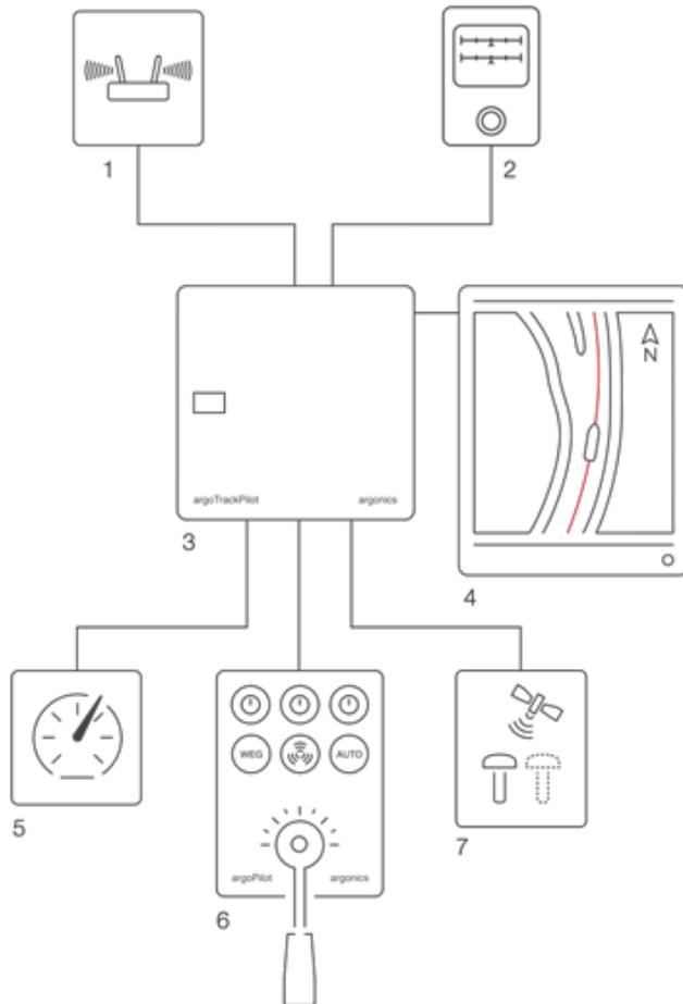
**Figure 2: Functional drawing of the AlphaRiverTrackPilot**
