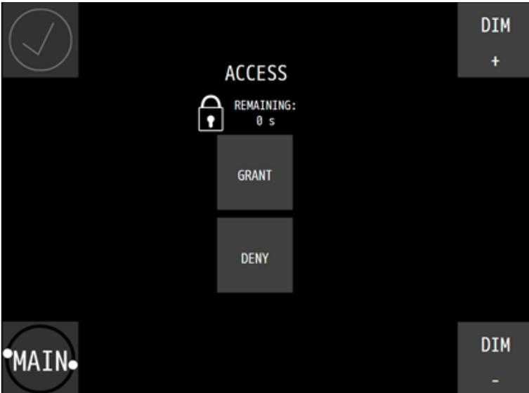
**GRANT:** Pressing this button opens the access for external connections. This is important for remote maintenance and updates done by support.
