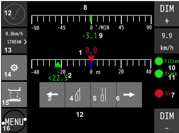
1. **Current** offset (Distance between original guiding line and parallel line): The blue line at 0.0m offset corresponds to the original guiding line. The red label displays the current offset. If the red label is to the left of the blue line, the ship will move at the desired offset to the port side of the original line, and vice versa.
