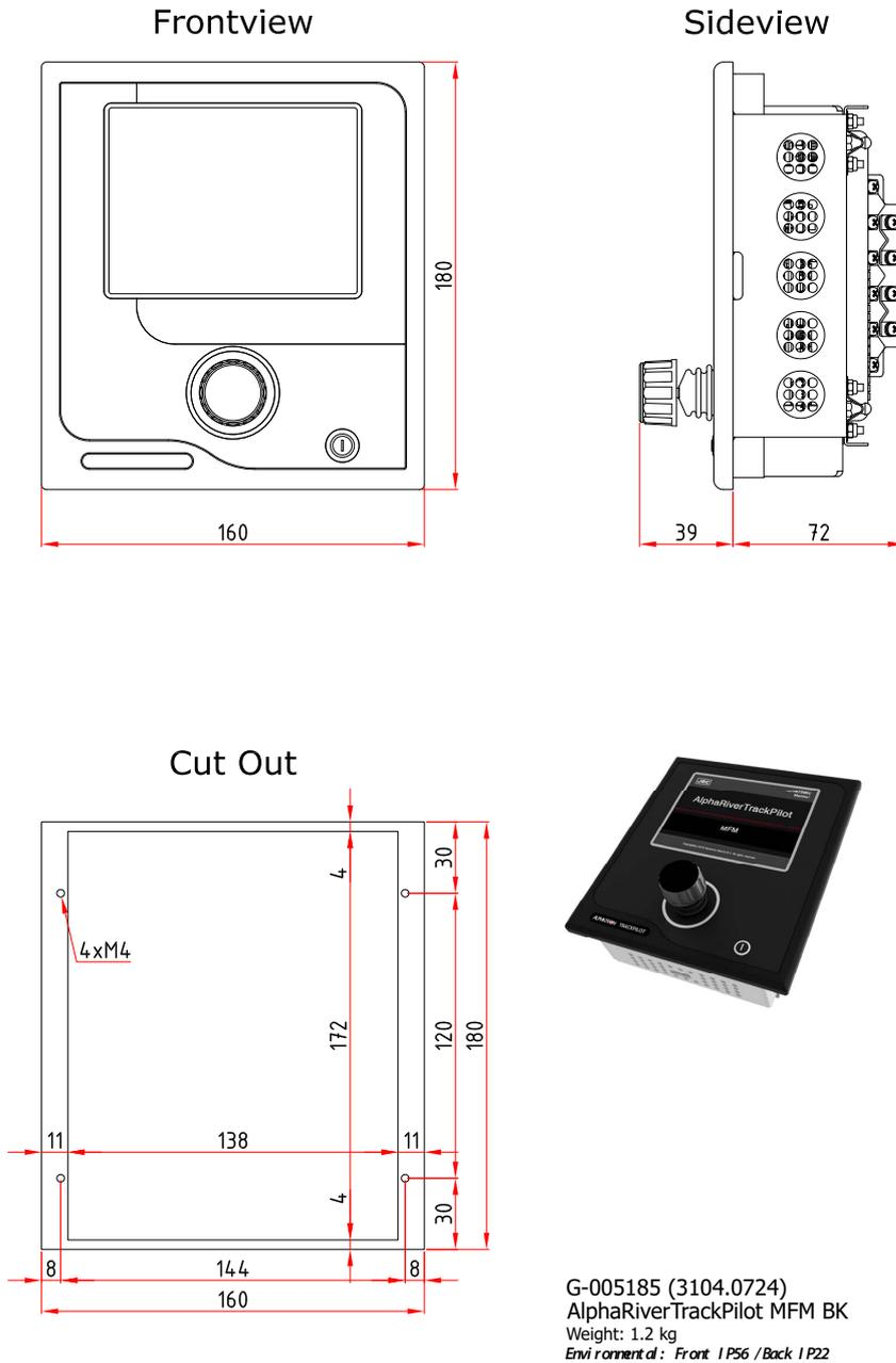
Figure 6: Dimensions of the AlphaRiverTrackPilot
