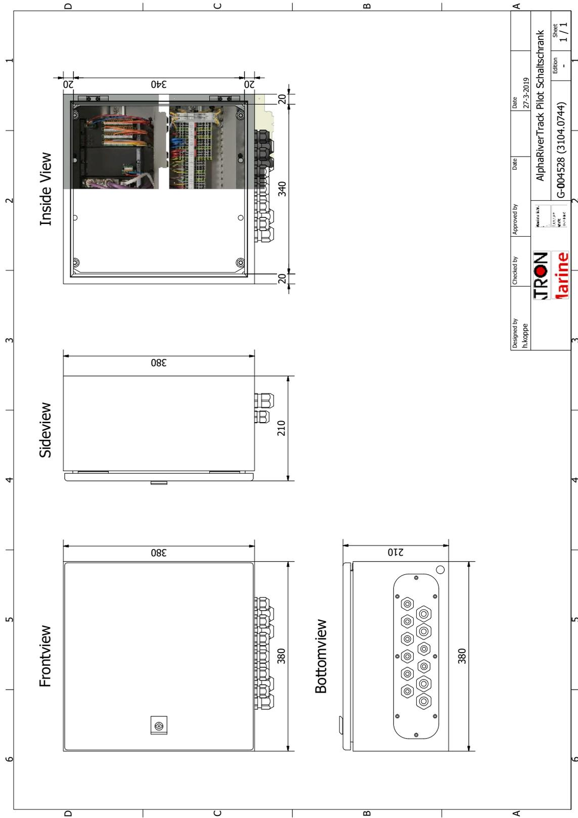
Figure 7: Dimensions of the control cabinet
