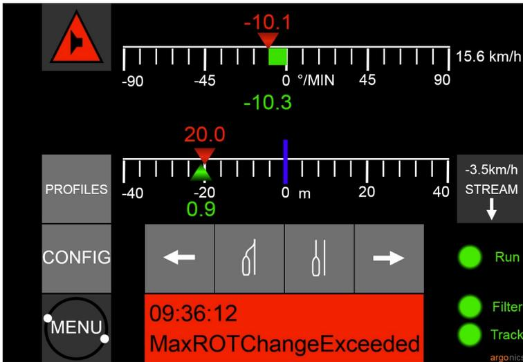
**!** **Important** Alarms can only be reset, by deactivating the TrackPilot.
