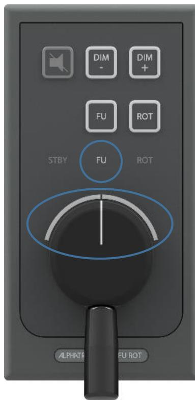
Figure 2: FU mode enabled
