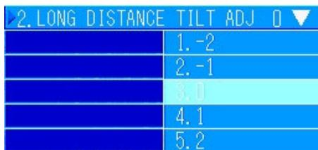
In the pulldown menu, you can set "-2 to 2". Set "5. 2" to automatically lower the tilt angle. Conversely, set "5. -2" to lower the tilt angle to 3° for surface schools of fish that are far away.
