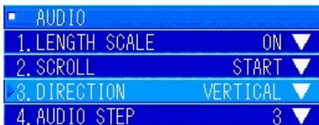
Turn the [MULTI] knob to select "3. DIRECTION". Press the [MULTI] knob to display the pulldown menu.
