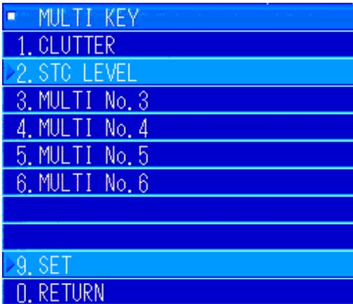
Turn the [MULTI] knob to move to "9. SET" and press the [MULTI] knob to complete registration.
