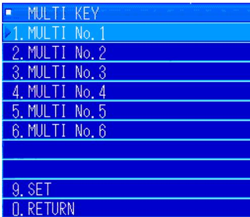
Turn the [MULTI] knob to move to "1. MULTI No.1" and press the [MULTI] knob to set "1. CLUTTER".
