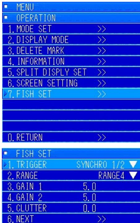
Press the [MENU] key to display the menus. Turn the [MULTI] knob to select "8. OPERATION" and press the [MULTI] knob to open the submenu. In the submenu, turn the [MULTI] knob to select "7. FISH SET".
