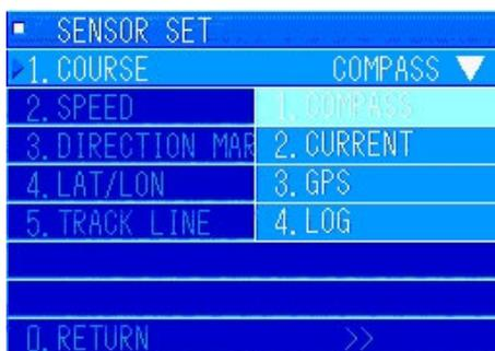
In the [SENSOR SET] menu, turn the [MULTI] knob to select "1. COURSE". Press the [MULTI] knob to display the pulldown menu.
