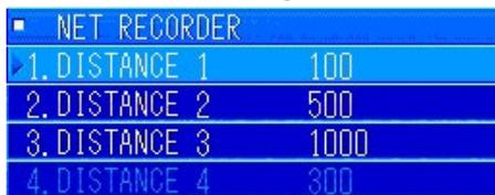
In the [NET RECORDER] menu, turn the [MULTI] knob to select "1. DISTANCE 1". Press the [MULTI] knob to display the menu for inputting values.
