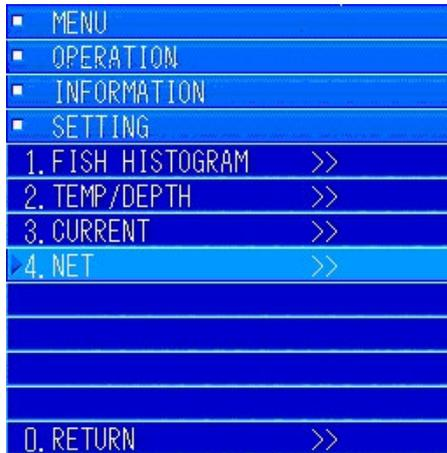
Follow the menu operations for setting display to display the "SETTING" submenu.
