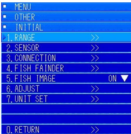
Open the "1. INITIAL" menu. Turn the [MULTI] knob to move to "1. RANGE", and then press the [MULTI] knob to open the submenu.
