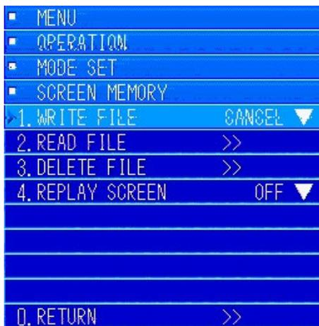
Turn the [MULTI] knob to select "1. WRITE FILE". Select "2. WRITE FILE" from the pulldown menu, and then press the [MULTI] knob to start saving.
