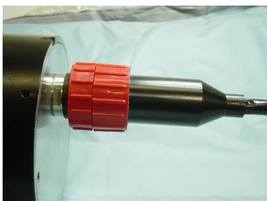
Figure 17. Connect cable and locking ring
