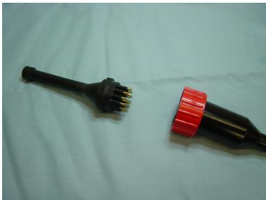
Figure 9. Remove connector cap from cable
