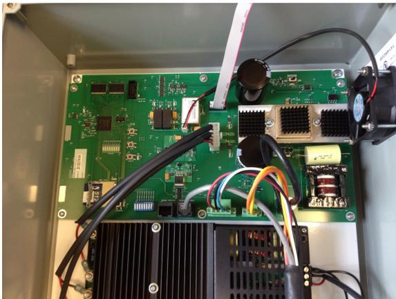
*Figure 6. Minimize strain on wires - bulkhead mount Power Module*
