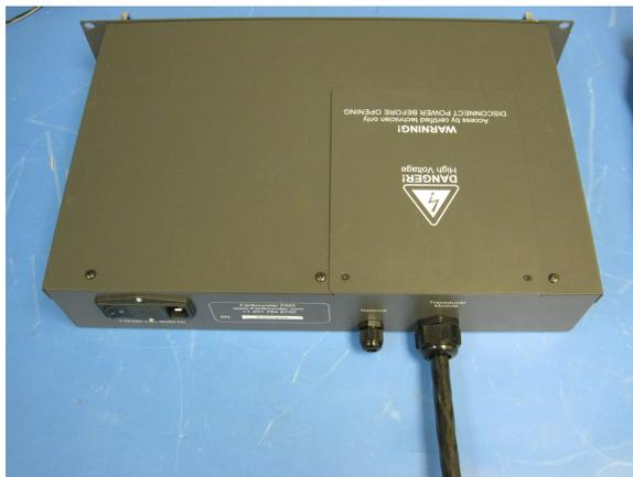
Figure 20. Transducer Module Connection Cable entry into rack mount Power Module
