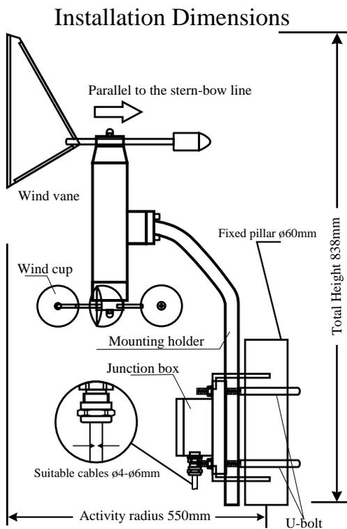
**Figure 2: Installation of anemometer**
