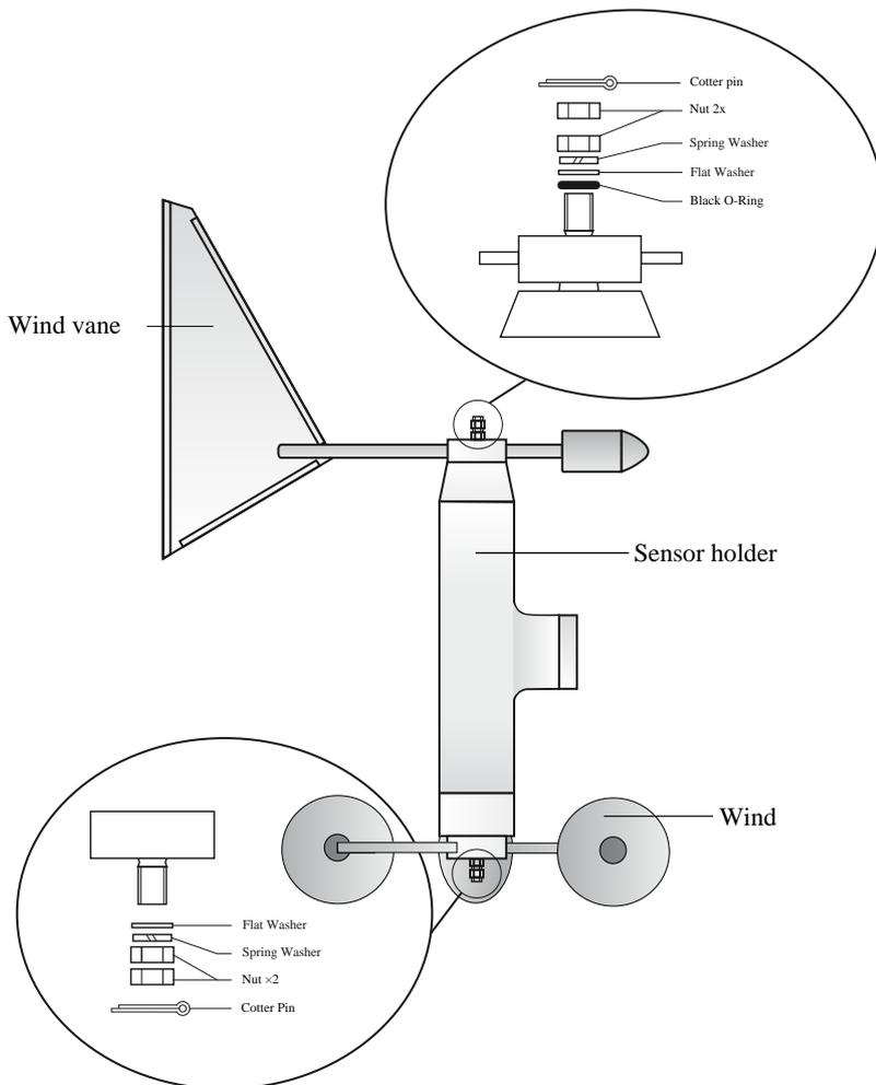
Figure 1: Installation of wind vane and wind cup
