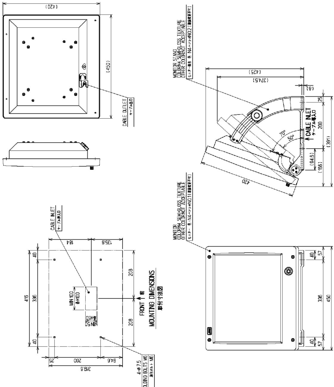
**Fig. 1.7 Outside Drawing of NWZ-173 LCD MONITOR with MPBC42446 STAND (Option)**
