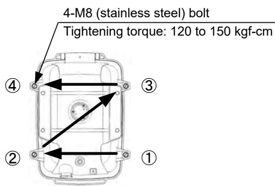
Bolt Tightening Procedure of
