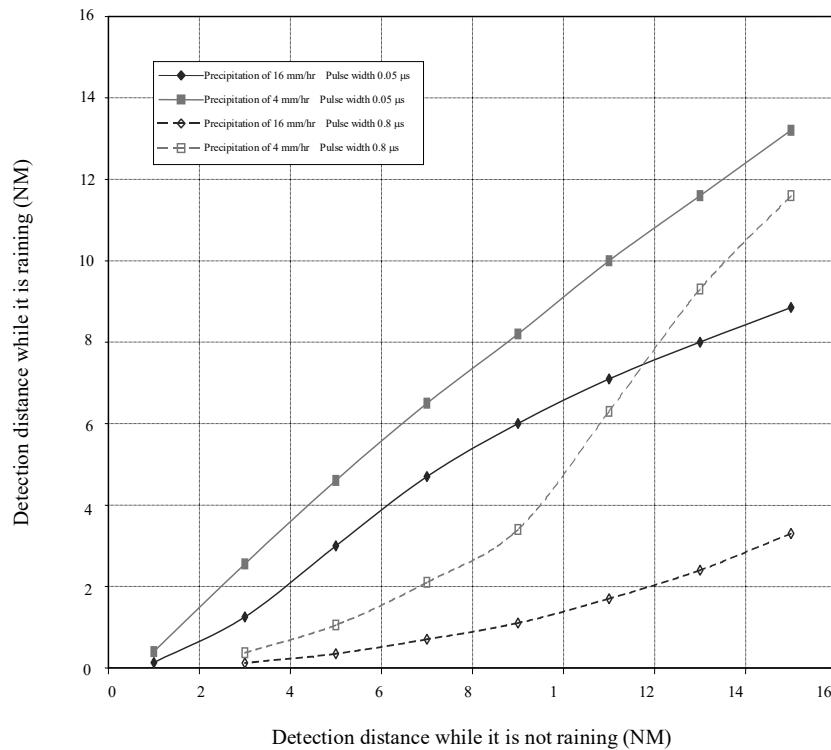
**Figure 6.5 Decreased target detection distance by X band radar due to precipitation**
