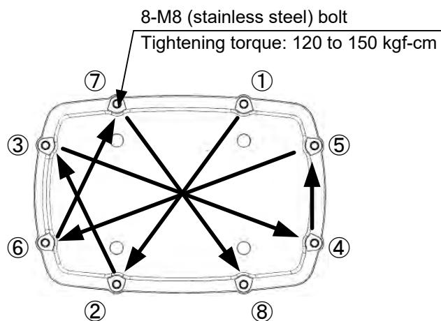
Bolt Tightening Procedure of
