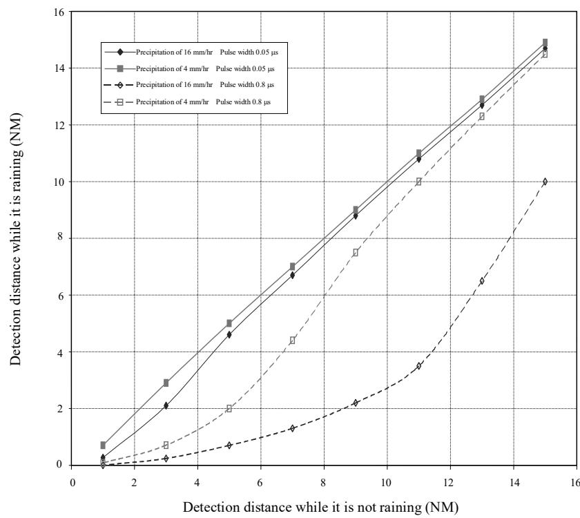
**Figure 6.4 Decreased target detection distance by S band radar due to precipitation**
