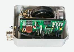
The Basicturn has a galvanic separted signal output that can be connected for example to the turn indicator on the radar monitor. It has an output as well for the autopilot. Apart from this, the Basicturn has an alarm output showing whether the turn indicator is in alarm mode.
