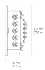
8.4-inch touch display 800-by-600-pixel resolution Horizontal orientation 450 cd/m2 max brightness View angle (H/V) 170° Panel cutout 216x172 mm
