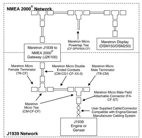
Figure 5 – Single Engine/Genset, No J1939 Network Installation Diagram
