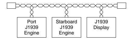
Figure 3 - Two Engine, Single J1939 Network
