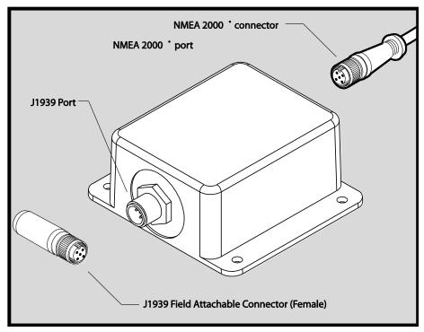
Figure 2 - J2K100 Electrical Connections
