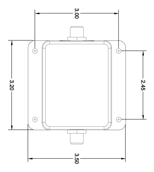
Figure 5 – Mounting Surface Template
