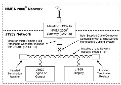
Figure 6 – Single Engine/Genset, Single J1939 Network Installation Diagram
