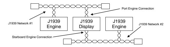
Figure 4 – Two Engines, Dual J1939 Networks
