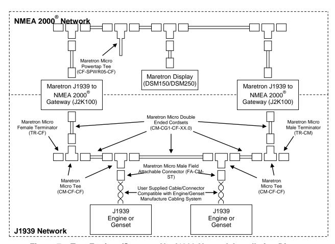
Figure 7 – Two Engines/Gensets, No J1939 Network Installation Diagram
