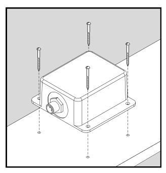
Figure 1 – Mounting the J2K100
