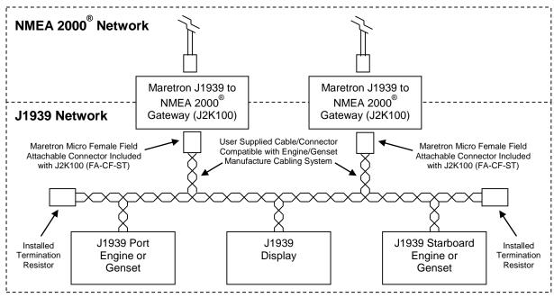
Figure 8 – Two Engines/Gensets, Single J1939 Network Installation Diagram
