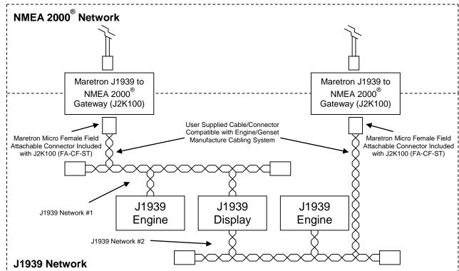
Figure 9 – Two Engines/Gensets, Dual J1939 Network Installation Diagram
