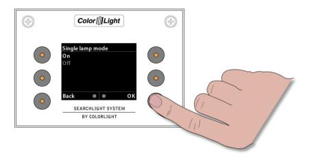
By selecting single lamp mode "On" and confirm by pressing "OK", the left bulb will turn on / off by pressing the left light button (2) and right bulb on / off by pressing the right light button (5).
