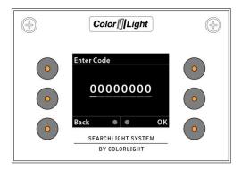
The code is entered by moving the joystick up and down to select correct character. To move to next character the joystick is moved to the right. Finish the process by select "**OK**" by pushing the button at the right bottom corner of the display
