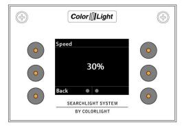
To change the speed move the joystick up or down to desired speed, press "**OK**" to update the searchlight with the new speed.
