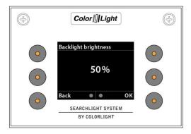
In this menu the light intensity of the button LEDs and display is set.
