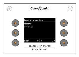
Some operators want to have their joystick to move the lamp housing vertically in the same direction as the joysticks physical direction:
