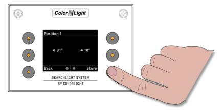
To set a position, enter the desired position, then move the searchlight to the by using the desired position by the joystick. Press "**Store**" to store each position.
