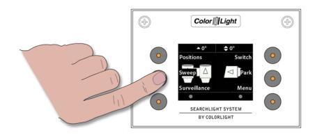
To enter the "Sweep" submenu, open up the quick start menu and press the left middle button "Sweep".
