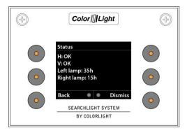
This menu will give information in form of text messages if there is errors.in the system, it also contains a "**bulb life**" counter showing total burning time in hours.
