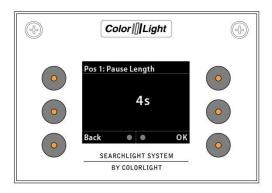
After pressing "Store" a new menu will appear, "Pause Length". This defines how long the searchlight will rest at this position before starting to move to the next position. Pause length can be set between zero and ten seconds.
