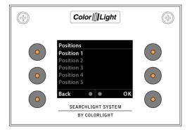
To set the positions in a surveillance sweep enter the "**Positions**" menu in the "**Surveillance**" submenu.
