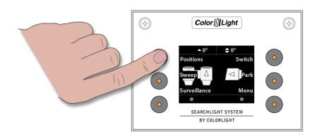
To enter the "Fixed Light Position" submenu, open up the quick start menu and press the upper left button "Positions".
