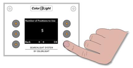
Select the requested number of positions (max. five) to be used in this surveillance sweep. Press "**OK**" to save and return to the "**Surveillance**" submenu.
