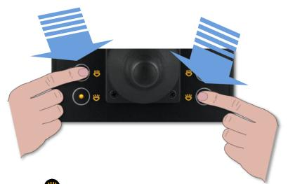
Pressing the spot buttons changes the focus towards spot on corresponding lamp house in predefined steps according to table above.
