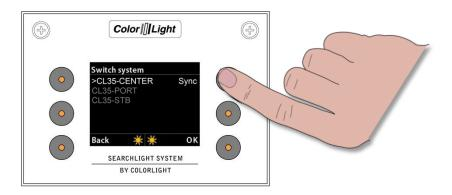
Once you have switched over to the searchlight which you want to be master in the system, press the "**Sync**" button, In this case, we choose CL35 CENTER as our master. The arrow in front of the selected CL35 CENTER tells us that this system is the "master" in the network and if the sync function is activated all the slaves will follow the masters movement.
