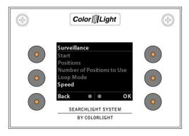
"**Speed**" is where the speed of the rotation of the searchlight is set. Default setting is 50% of maximum speed of the searchlight.
