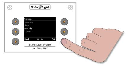
To modify the sweep angle and / or the center of the sweep enter the "Sweep" menu and navigate down to "Modify", press "OK".
