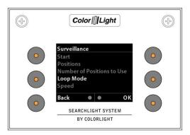
Surveillance has a couple of different settings, "Loop Mode" and "Speed". In "Loop Mode" there are two choices, "Back and Forth" and "Repeat".
