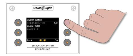
Add or remove one or more slaves is done by entering the "switch" submenu and with the joystick scroll through the list of available headlights, If the searchlight in the list is not connected in the synchronized group control, the text "Add" appears next to the top left button, to add this searchlight to the group, press the "Add" button.
