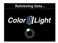
At system startup, the panels will start to scan the network to find connected electrical boxes, during this time, the panel software version will be displayed.
