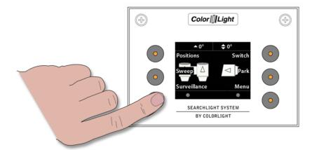
To enter the "Surveillance" submenu, open up the quick start menu and press the bottom left button.
