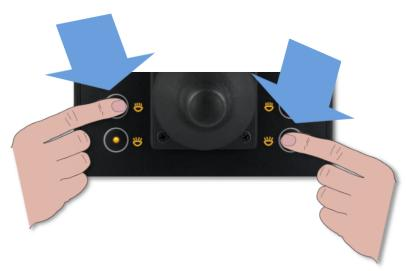
Pressing the focus buttons (3) or (4) changes the focus for the left lamp house and buttons (6) or (7) changes focus for the right lamp house.
