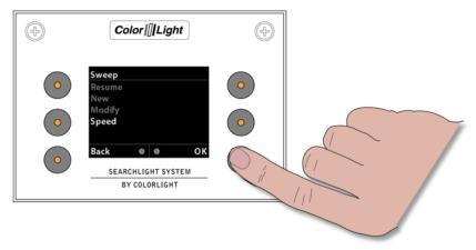
The default speed of the sweep is set to 50% of the maximum speed of the searchlight. To change the speed of the sweep enter the "**Sweep**" menu and navigate down to "**Speed**". Press "**OK**" to enter the "**Speed**" submenu.
