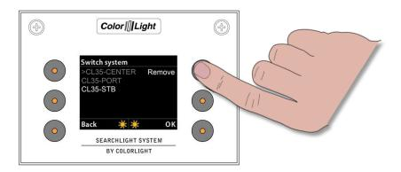
If the searchlight marked is already listed as slave in the group, the text "**Remove**" appears next to the top left button, to remove this searchlight from the group, press the "**Remove**" button.
