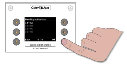
There are up to four fixed position memories (**A**, **B**, **C** and **D**) which can be individually programmed.
