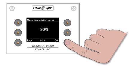
The adjustment is done by moving the joystick forward to change speed in increments of 5% and backwards to decrease. Minimum speed is 20% and maximum 100%, when the choice is confirmed with "**OK**", the display jump back to the previous "**Settings**" - menu.
