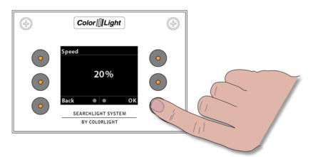
Change the setting by moving the joystick up or down in the speed menu until the requested value is shown. The speed can be set between 5-100% of the maximum rotation speed.
