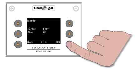
This menu changes the sweep angle and center point of the sweep, modification can be carried out both during movement and while searchlight is standing still.
