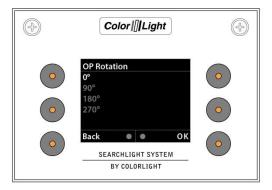
By changing this setting you can compensate for different mounting positions while maintaining accurate indicator function, you can choose from four different positions.
