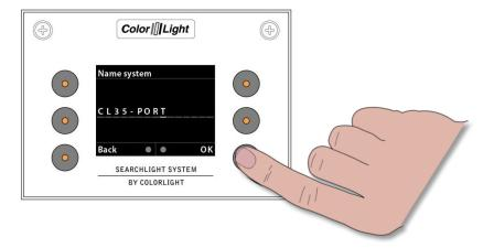
The name is set by moving the joystick up and down to select correct character. To move to next character in the name the joystick is moved to the right. Finish the name process and save the name by select "**OK**" by pushing the button at the right bottom corner of the display.
