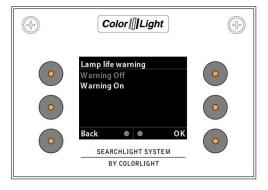
"Lamp life warning" menu will make it possible for the operator to choose if the lamp life warning feature should be activated or not. See 8. SWITCH ON LIGHT. The warning is normally enabled when system is shipped from ColorLight.
