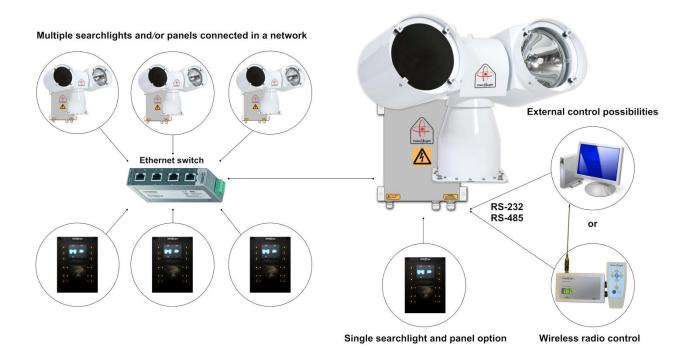
ColorLight has with its newly developed control system for searchlights opened for a flexible and future-proof system in which several searchlight assemblies (CL20, CL25 and CL35) and operator panels can be connected to a <u>dedicated</u> network and communicate via the Ethernet infrastructure.
