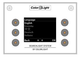
The language in the display can be changed depending on which language sets that are installed in the operator panel.
