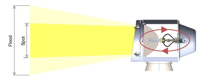
As long as a focus button is pressed the bulb moves in and out which changes the focus of the light between 4-20 degrees for model CL20, CL25 and 3-20 degrees for model CL35.
