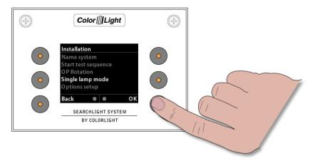
Normally, for double white (CLXX-11) or double UV (CLXX-22) configuration one wants to ignite both bulbs simultaneously and thereby obtain maximum light intensity with the push of a single button.
