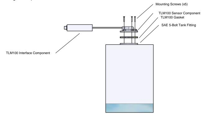
Figure 2 – TLM100 Mounting – SAE 5-Hole Bolt Pattern
