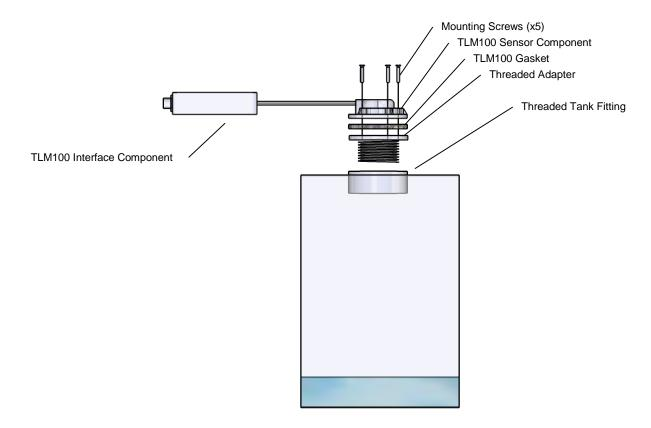
Figure 4 – TLM100 Mounting With Threaded Adapter
