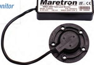
The TLM100 is mounted directly to the top of tanks using the industry standard SAE J1810 5-hole mounting pattern. The TLM100 can also be mounted to tanks with threaded tank openings using optional adapters that included both a 1.5" NPT and a 1.25" BSP adapter. There are other important TLM100 optional accessories including an optional focus tube to permit use on boats with planing hulls, which is required if the vessel spends a significant amount of time with the bow pitched up.
