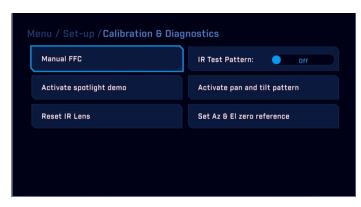
**Manual FFC** This function applies to the IR camera only. When selected, the camera drives the camera to a preset position and performs the FFC calibration (< 5 s). The camera then returns to its Home position.
