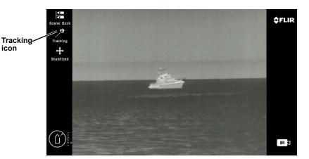
**Tracking state**—When the target is acquired, the acquisition gate disappears and the tracking icon is shown.
