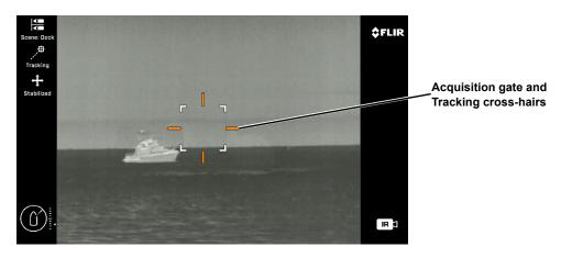
Joystick Buttons: Left - Cancel tracking to reacquire target Right - Reacquire target
