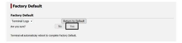
JUE-60GX starts in the factory default setting when the machine is Automatic restarted.
