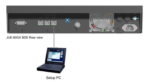
Set the IP address of the PC. Under the factory default settings, JUE-60GX is set as follows.
