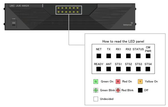
The shapes and precise colors of LED are different from the actual shapes and colors.
