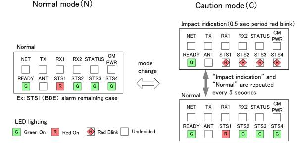
Please note the caution mode behavior is different before and after the accumulated-time-threshold (ACC-th) is exceeded.
