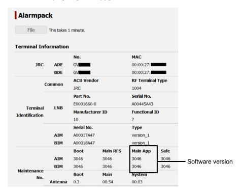
If the same number as "xxxx" of the software file, [JUE-60GX\_PKG\_xxxx.jrc], is displayed, the software has been upgraded correctly.
