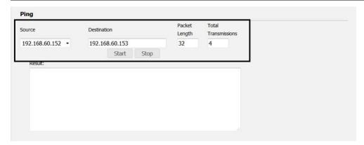
1 Enter the IP address of the transmission source in [Source].
