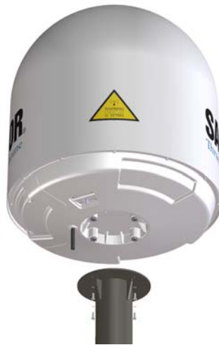
Figure 3-17: Mounting the ADU on the mast flange
