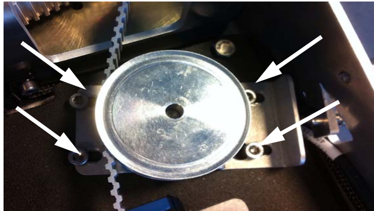
Figure 8-48: Azimuth motor, tighten the belt tensioner
