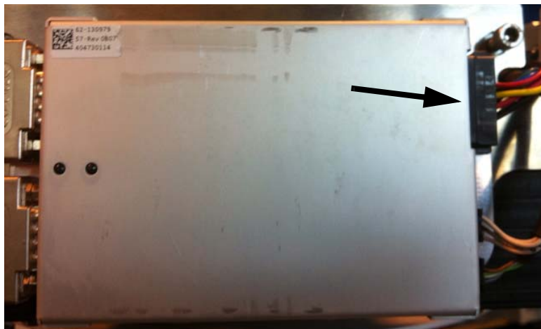
Figure 8-44: Azimuth DDM, disconnect connector
