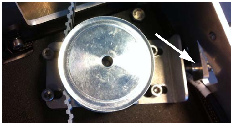
Figure 8-53: Azimuth Encoder, adjust belt tension
