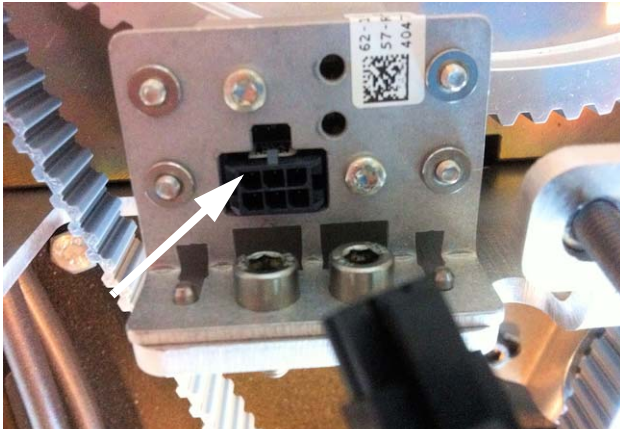
Figure 8-74: Azimuth ZRM, disconnect connector
