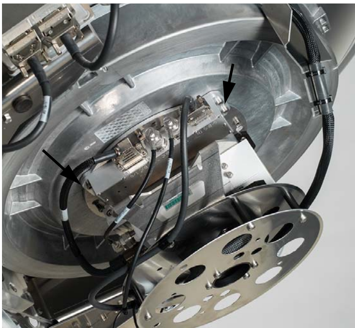
Figure 8-33: Cable connection from the cable wrap
