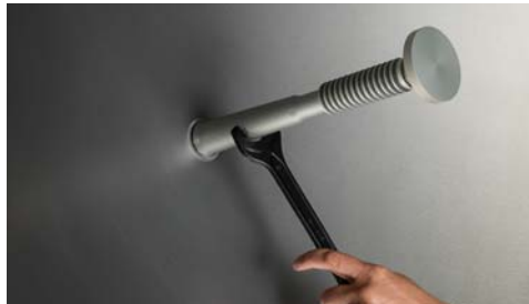
Figure 8-76: Removal of the Ka feed horn
