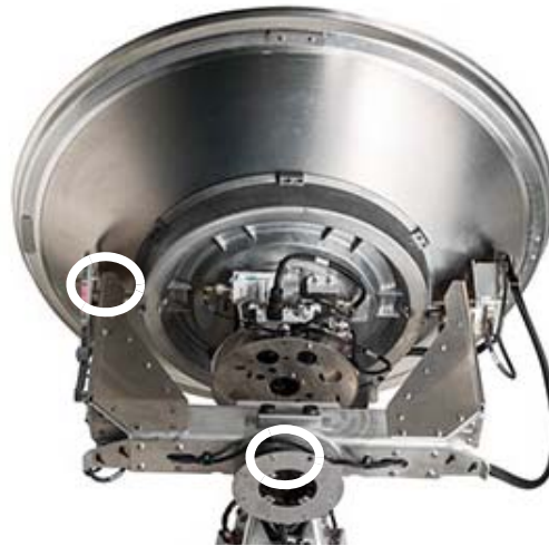
Figure 8-67: Location of the Zero Reference Modules (ZRM)
