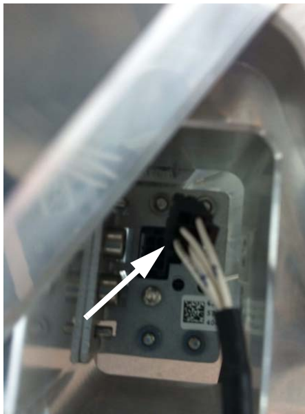
Figure 8-69: X Elevation ZRM, disconnect connector
