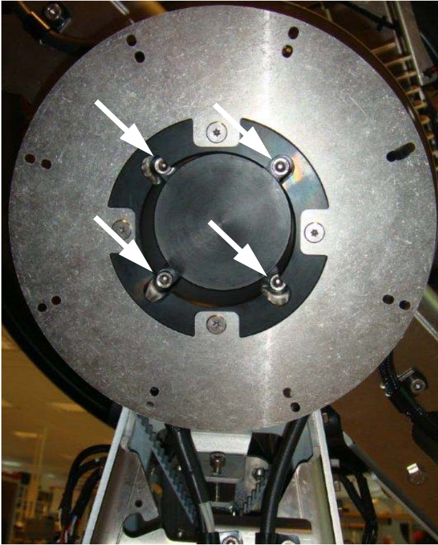
Figure 8-61: Removing the cable drum
