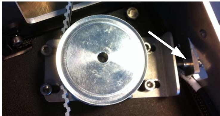
Figure 8-52: Azimuth encoder, adjust belt tension
