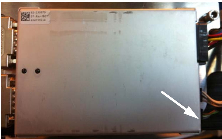
Figure 8-50: Azimuth DDM, disconnect connector
