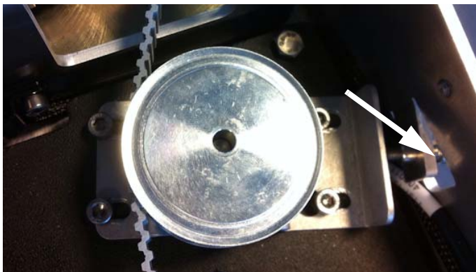
Figure 8-47: Azimuth motor, adjust belt tension
