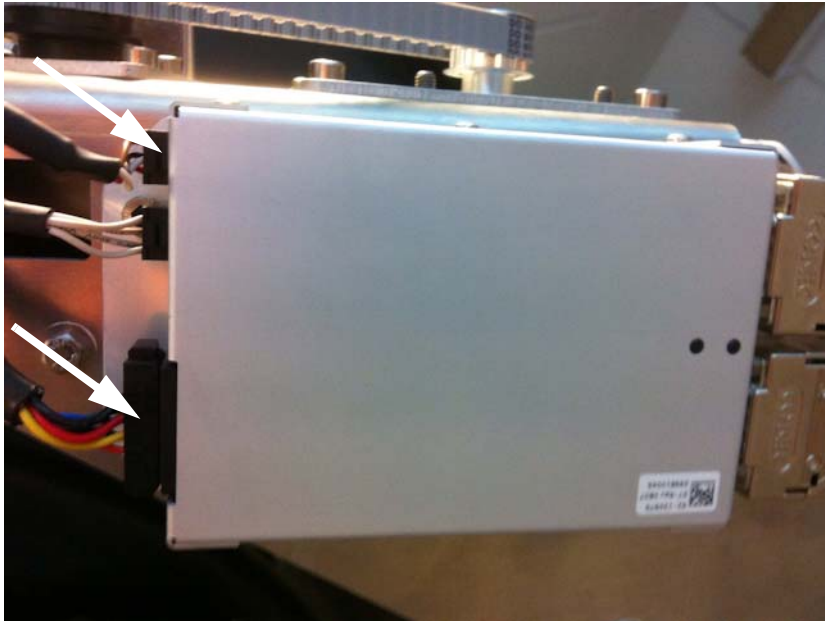
Figure 8-37: Elevation DDM, disconnect 2 connectors
