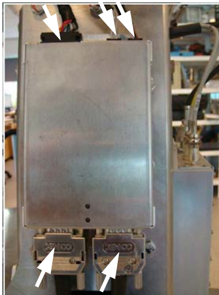
Figure 8-28: Replacing the DDM — remove connectors
