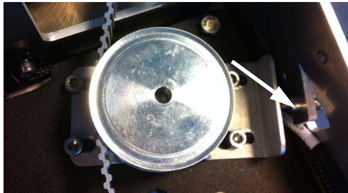
Figure 8-64: Azimuth drive belt, adjust belt tension
