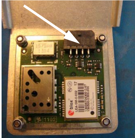
Figure 8-20: Connector for GPS PCB
