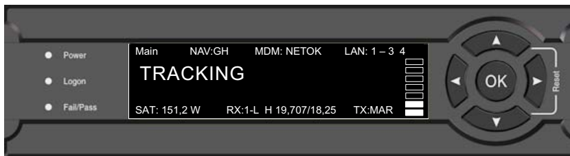
Figure 4-1: ACU: LEDs, display and keypad (detailed, example)
