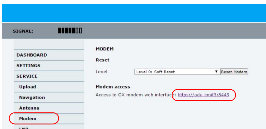
Figure 6-10: Web interface: SERVICE > Modem, Factory default
