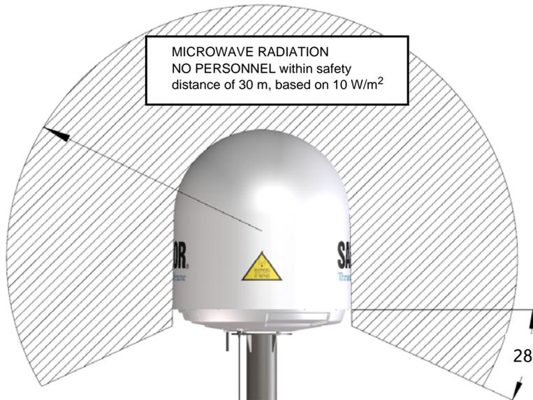
Figure 3-4: Radiation hazard, safety distance 30 m
