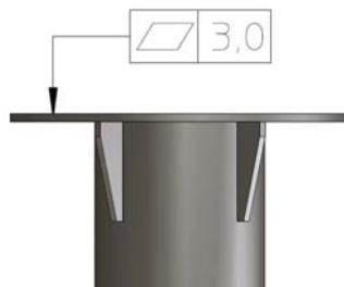
Figure 3-7: ADU mast flange, recommended flatness on the mast mount plateau
