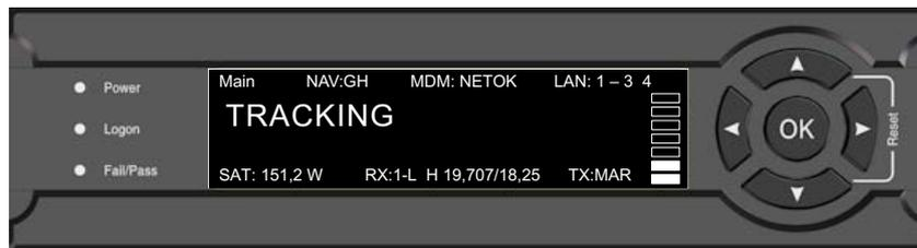
Figure 4-1: ACU: LEDs, display and keypad (detailed, example)
