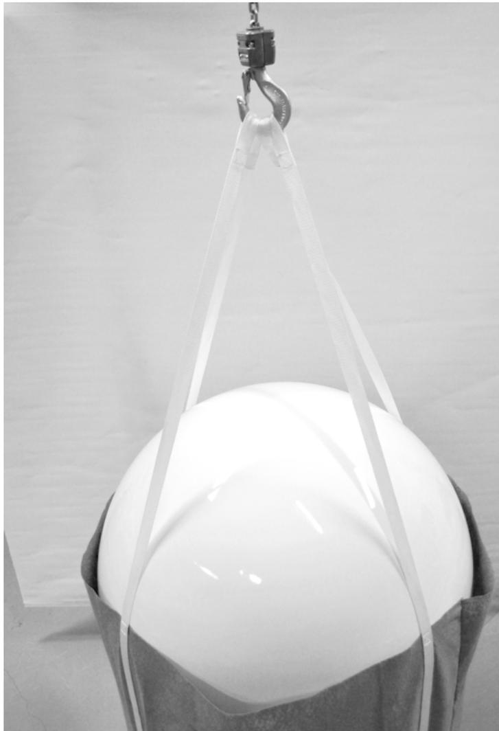
Figure 3-19: ADU installation, 4 lifting straps on crane hook
