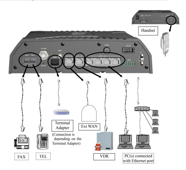
Fig.4.1.1 The Cable connection of each terminal
