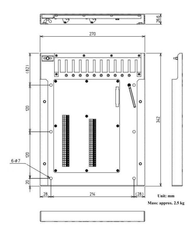
**Fig. 2.4.6** Appearance of Junction Board (CQD-2243)
