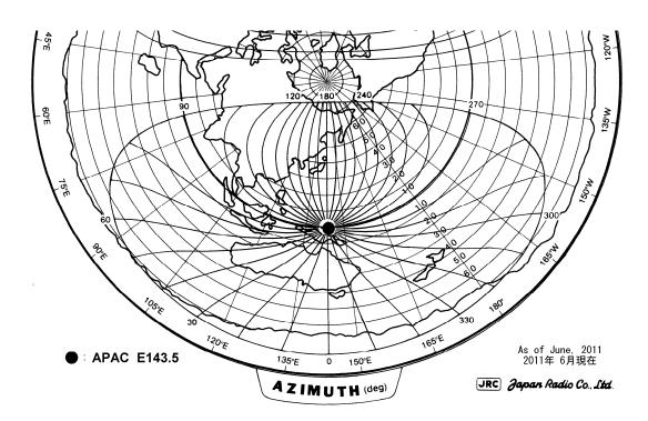
Fig.Q.2.4 Equal AZ line for APAC E143.5
