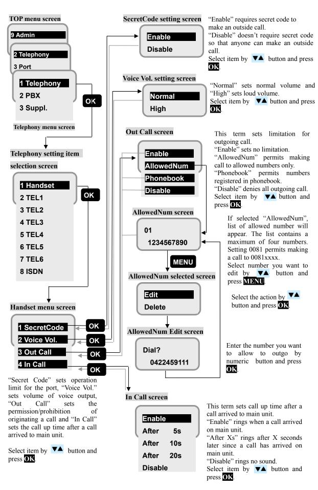
Fig 7.9.2.1a Flow of port setting (Handset)
