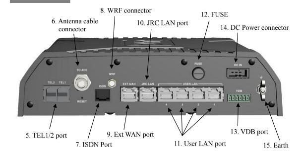
Fig. 3.2c Main unit rear view
