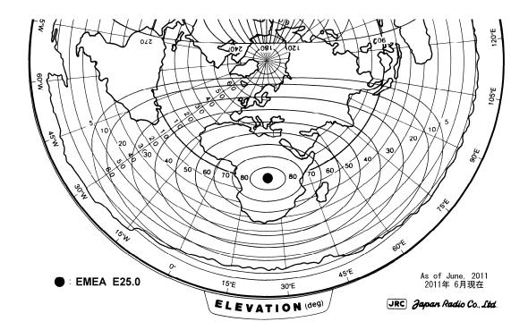
Fig.Q.2.1 Equal EL line for EMEA E25.0
