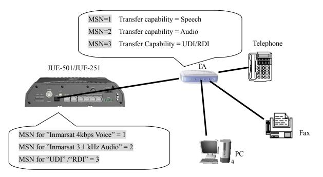
Fig.8b Connection sample of ISDN port
