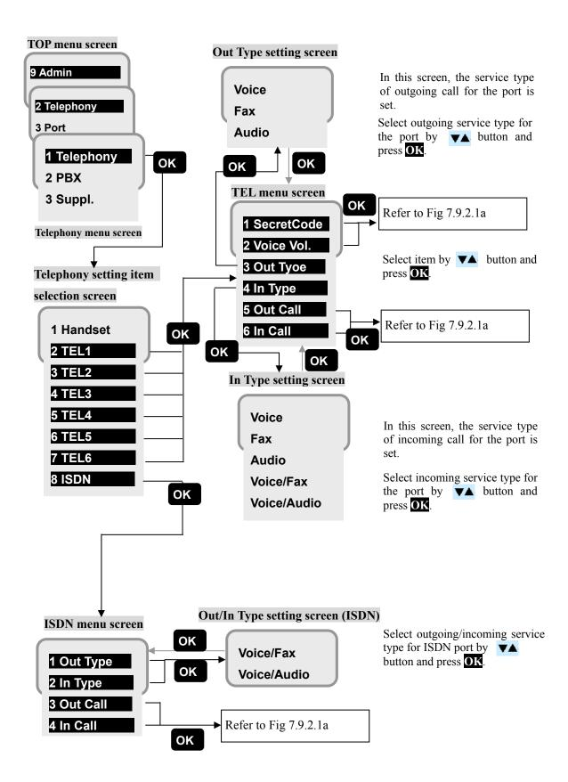
Fig 7.9.2.1b Flow of port setting (TEL ports and ISDN port)
