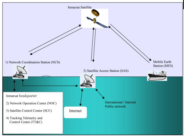
Fig.1.1.2 The Inmarsat FleetBroadband service Network
