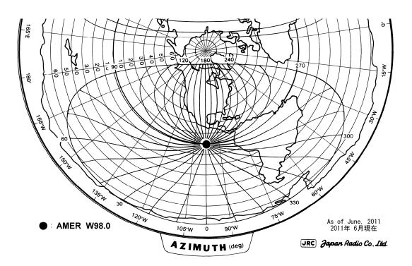
Fig.Q.2.6 Equal AZ line for AMER W98.0
