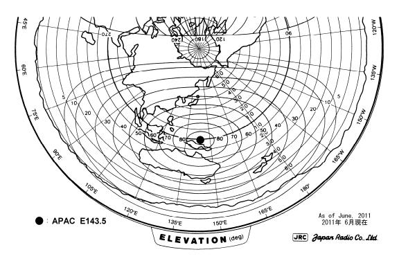
Fig.Q.2.3 Equal EL line for APAC E143.5
