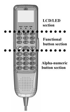
Fig. 3.4b Section of Handset
