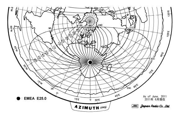
Fig.Q.2.2 Equal AZ line for EMEA E25.0
