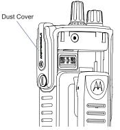
Insert the hooked end of the cover into the slots above the universal connector. Press downward on the cover to seat the lower tab properly into the RF connector.
