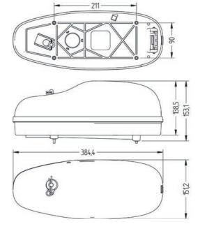
chemicals, oil, exhaust and vibrations. The braket shall be mounted as high as possible, but fullfill the above requirements. This will ensure operation of the hydrostatic float-free release unit, in the event of the vessel capsizes without sinking.
