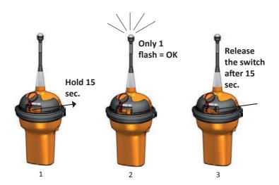
**Note:** Tests should be limited to the first five minutes of the hour, as the satelite EPIRB emits a 121,5 MHz singla during test.
