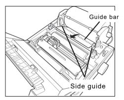
Insert the leading edge of the paper into the rear of the platen. Then turn the paper feed knob to feed the paper out and adjust the direction.
