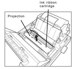
Lusing the knob on the new cartridge make the ribbon taut. Then manually move the print head to the left edge, and attach the ribbon with such a pen so that it is between the ribbon mask and print head.
