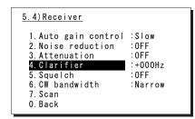
Press ENT to move the cursor to the right, then use the jog dial or numeric keypad to select a value in the range of -200 to +200 Hz.
