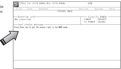
On the main menu and the dropdown menu, select System → NBDP setup with Enter key.
