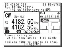
Communicate in CW mode using the CW keyer connected to the KEY jack on the controller as shown in the figure to the right.
