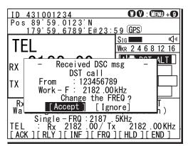
3. To acknowledge to the distress alert after coordination with the coast station, from the above right screen, press **FUNC** key to move the active screen to the message control area. Then select ACK with jog dial and press ENT to send the acknowledgement.
