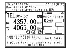
Pressing ENT causes the channel group number to blink so a channel group can be input.
