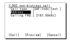
Press ENT on the Call to start sending the safety test call.
