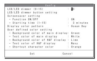
When completing the setting, move the cursor to the Set and press Enter key.
