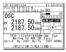
When the acknowledgement is received, the ALM lamp blinks and the alert starts sounding. After silencing it with CANCEL key, the screen becomes as shown at right.
