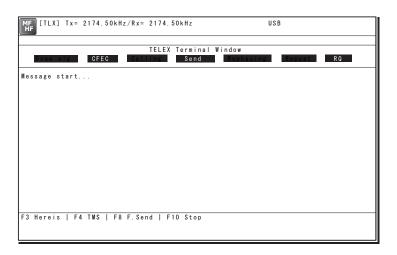
• The characters typed with the keyboard can be transmitted in sequence. And all of the characters displayed on the screen are printed out on the printer.
