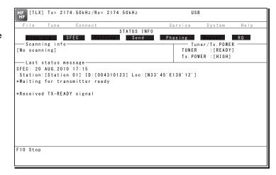
• After sending the phasing signal followed by the SELCAL number, the message sending using the SFEC mode will be available.
