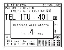
After the antenna is tuned, the distress alert is sent.
