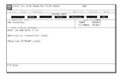
• After sending the phasing signal for about 15 seconds, the message sending using the CFEC mode will be available.
