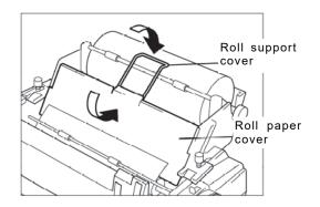
Close the printer cover, return the roll paper stand to its original position, and tighten the fixing screws.
