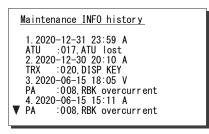
[Number] [Detection & recovery time] [A: Detection/V: Recovery] [Unit name]: [MI number], [Information]
