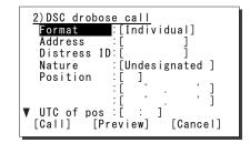
Select Address and press ENT, input the MMSI of the calling coast station.
