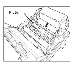
Restore the roll paper cover and the roll support cover as shown at right and close the printer cover.
