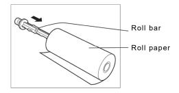
Pass the roll paper over the guide bar as shown in the figure at right.
