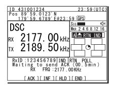
Additionally, note that if it is received while the 7.5.1.3 Polling call of the Automatic ACK menu is set to ON, and there is no active procedure, this call can be acknowledged automatically.
