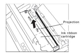
Using the knob on the new cartridge to make the ribbon taut, manually move the print head to the left edge, and attach the ribbon so that it is between the ribbon mask and print head.
