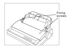
Pass the roll bar through the roll paper, and install the roll paper onto the roll paper stand paying attention to its orientation.
