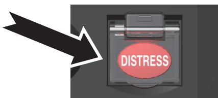
2. Press and hold the **DISTRESS** button for at least 3 seconds until the countdown is complete.
