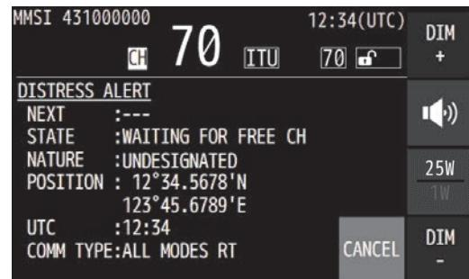
4. After sending the distress alert, wait for the acknowledgement in the condition of the activated distress transmission procedure.
