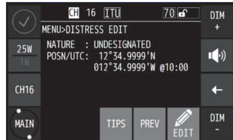
The nature of distress is set. If the position and time are not displayed automatically, select the [EDIT] → [POS UTC] buttons and input them manually.
