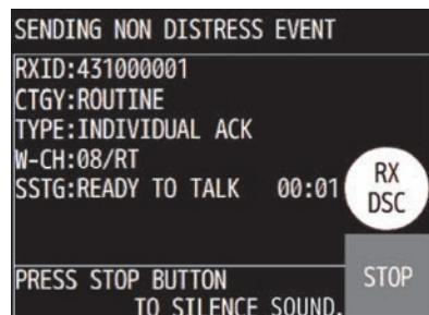
**5.** After setting the working channel, start communications using the handset.
