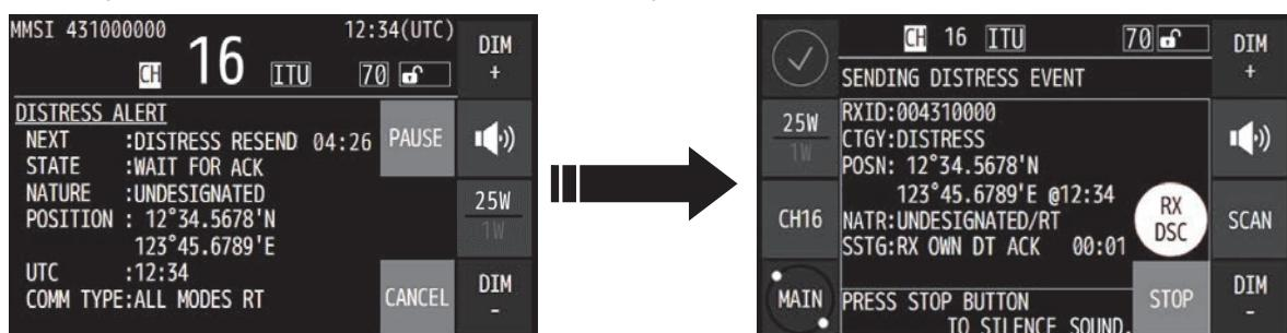
4. After receiving acknowledgement, lift the handset and request rescue using CH16 of the radiotelephone.
