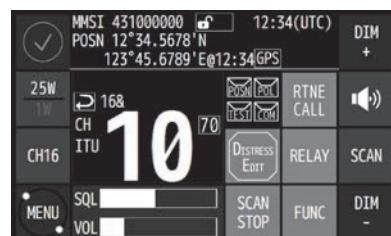
3. Touch the [SCAN STOP] button to stop scanning.
