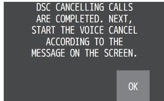
4. Touch the [OK] button and according to the guidance on the screen, broadcast to cancel the distress alert.
