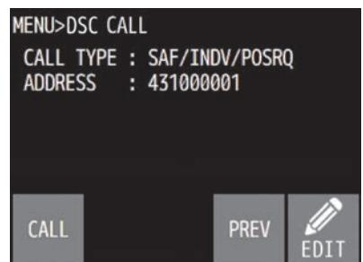
3. When acknowledgement is received, the RX DSC mark flashes and the alert sounds. After silencing it with the [STOP] button, a received screen as shown at right appears.
