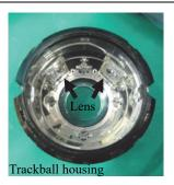
7 After cleaning them, reinstall the ball and the stopper ring. Don't forget to tighten the stopper ring.
