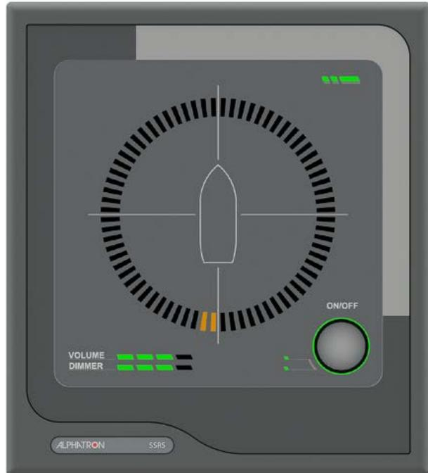
Figure 14: Selecting the Aft Microphone
