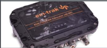
The B330 is a truly ruggedised device designed to operate reliably for years without maintenance in even the harshest external marine environment.
