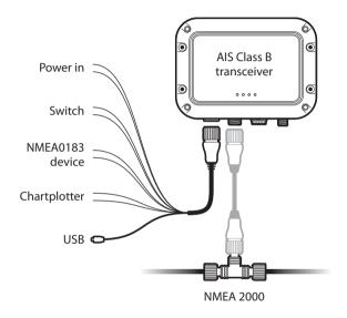
Figure 3 Electrical connections to the AIS transceiver
