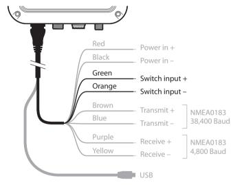
Figure 10 Connecting an external switch
