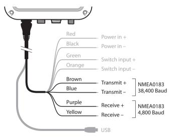
Figure 11 Connecting to the NMEA0183 data port
