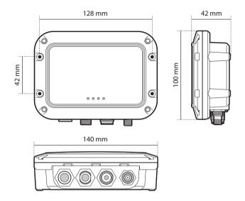
Figure 5 AIS transceiver dimensions
