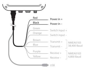
Figure 12 Connecting the power supply
