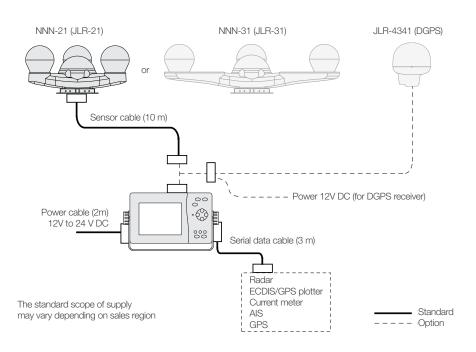
The maximum cable length between antenna and display is 50 m. Note that extensions should be of a shielded multicore cable to prevent noise or attenuation.
