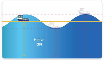
The JLR-21 has heave functionality built-in as standard. In rough ocean conditions (with high waves), the GPS compass can correct up and down (attitude), movement. This is especially useful for fish finders and sonars on fishing vessels where high waves are compensated for with up to 20 cm accuracy, providing better potential for a profitable catch.
