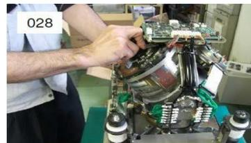
Tilt the Horizontal ring to the side where the connector is located. Carefully remove the defected Sensitive element as shown in above picture 028.
