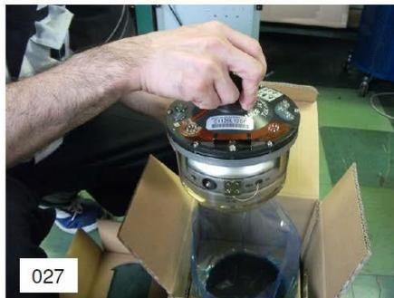
**Note** Handle Sensitive Element with great care. Do **NOT** tilt the element. It is filled with oil and the top is open.
