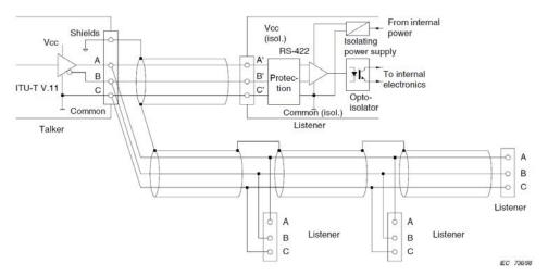
Figure 8: IEC 61162-2 Circuits
