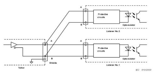
Figure 7: IEC 61162-1 Circuits
