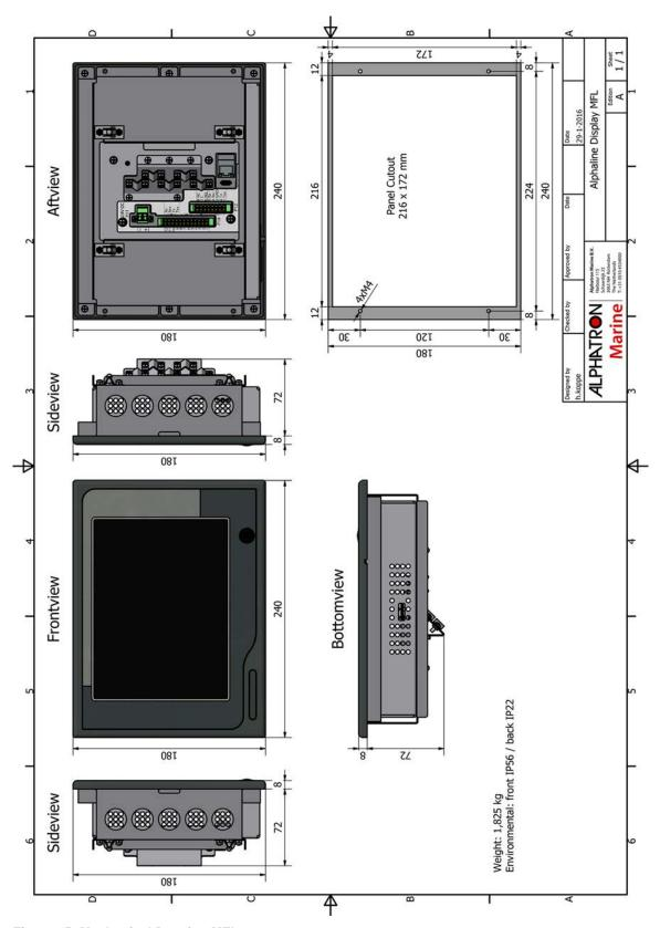
Figure 45: Mechanical Drawing MFL
