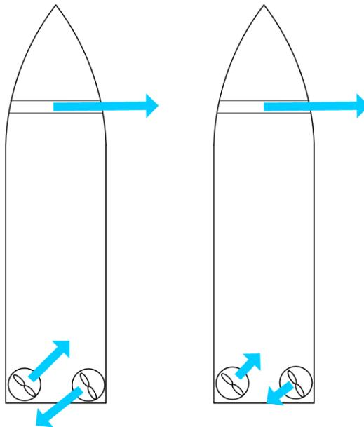
Figure 6.30: Thrust Allocation Modes: High and Low Bias
