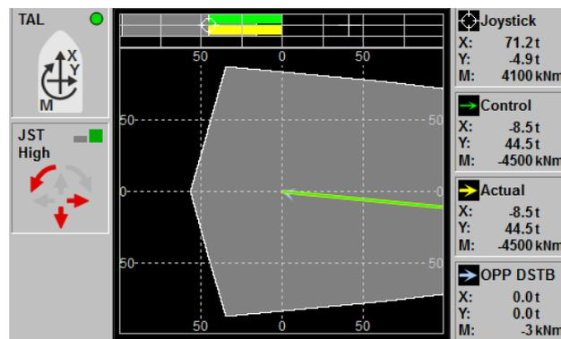
Figure 6.4: Thrust Ability Diagram. Red arrows: need to synchronize
