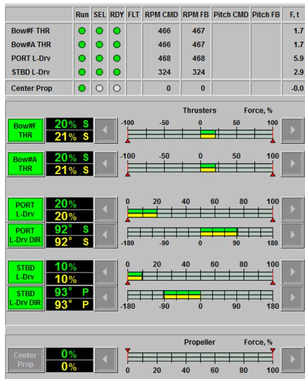
Figure 6.1: Manual Thruster Window
