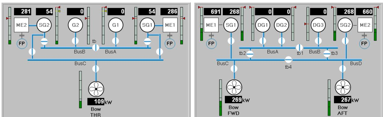
Figure 6.37: Power Mimic Diagram Examples
