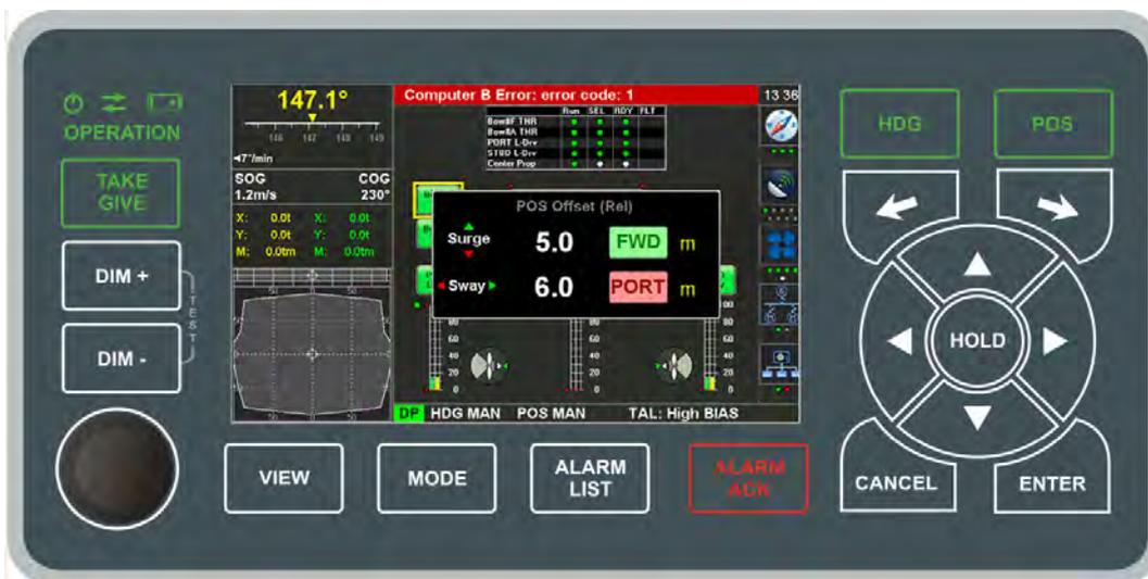
Figure 2.7: Control Panel Controls, Buttons and Indicators (MCP and PCP)
