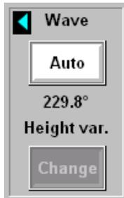
The value for wave direction is displayed under the **Wave** text in the **Auto** mode.
