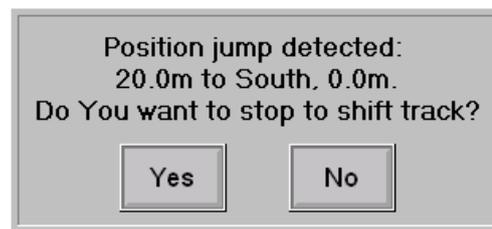
Figure 8.16: Dialog box in Low Speed Track Mode
