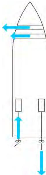
Figure 6.23: Thrust Allocation
