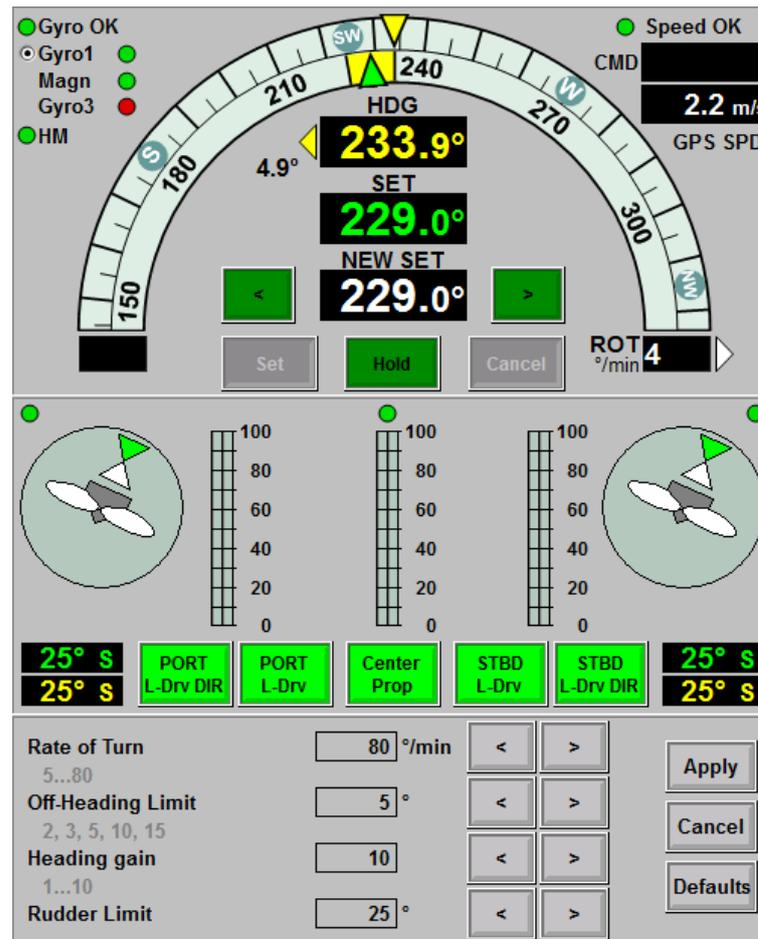
Figure 10.56: The Autopilot window with Monitor Heading indicator
