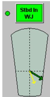
Figure 6.22: Waterjet thrust indicator
