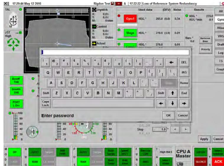
Figure 7.2: The password request for sensor parameters
