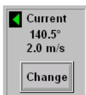
The values for current direction and speed set in the dialog box are displayed under the **Current** text.
