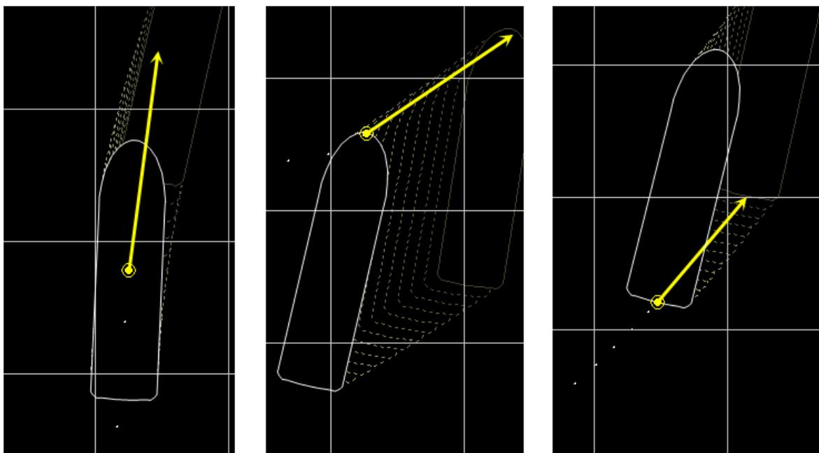
Figure 10.3: COR position: COR at Center, Bow, Stern
