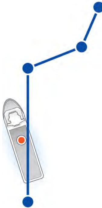
Figure 9.13: Position mode: LS Track Control
