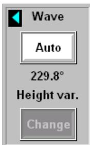
The present wave direction is displayed in degrees under the **Wave** text. It matches the wind direction in Auto mode.
