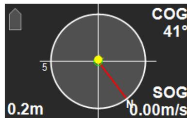
Figure 5.53: Position Console in the Hold Area Mode
