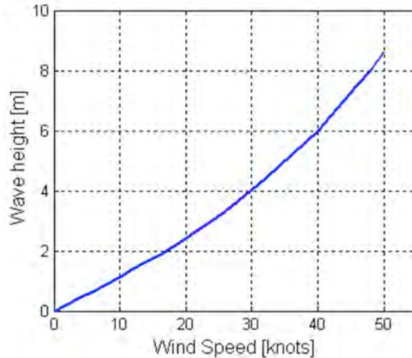
Figure 10.82: Relationship between Wave Height and Wind Speed
