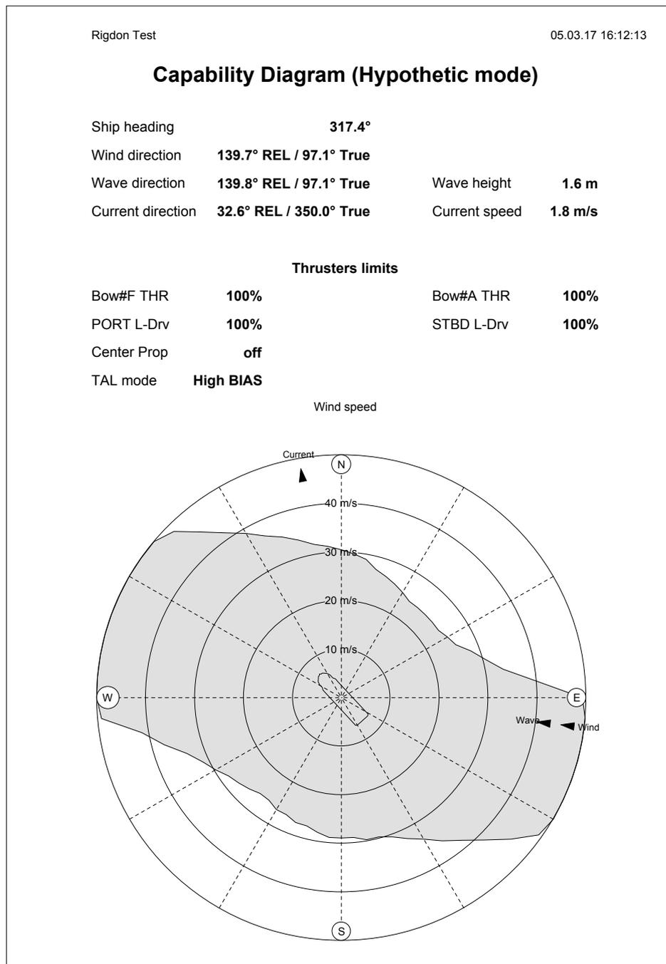
Figure 10.70: Example of the Capability Plot Printout (Hypothetic Mode, TRUE view)
