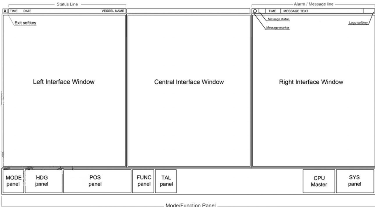
Figure 5.5: The Wide Screen Layout with Three Windows
