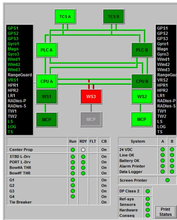
Figure 10.94: System Monitor Window Example — DP Class 2 System with 3 Workstations
