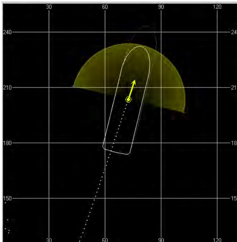
Figure 10.12: Map Window when the Min Power function is ON, and Sector parameter is ON
