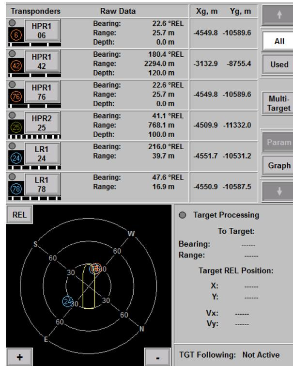
Figure 10.17: Target Window Example
