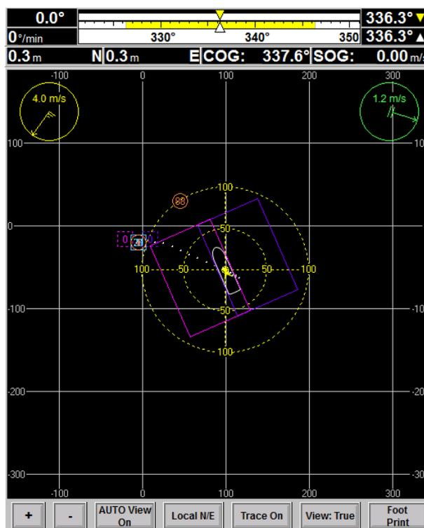
Figure 10.102: Map Window, "Foot Print" softkey is enabled
