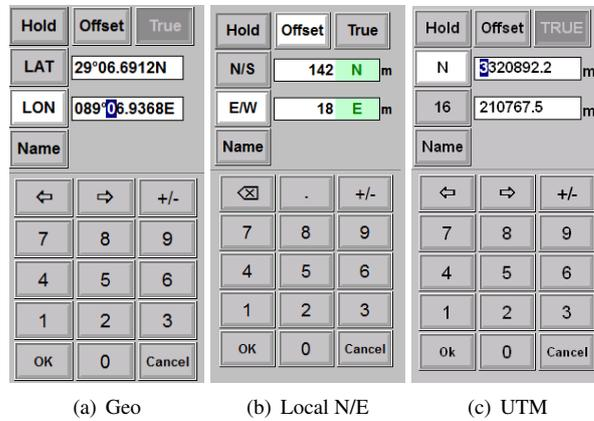
Figure 8.3: The waypoint set up dialogue for the different coordinate systems
