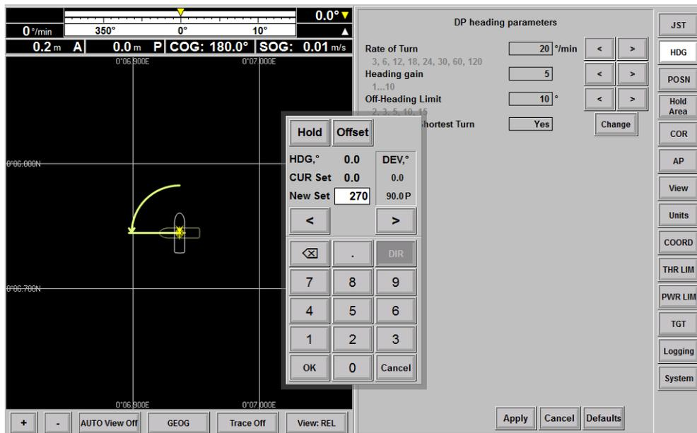
Figure 5.23: The turn track in case Always Use Shortest Turn=Yes
