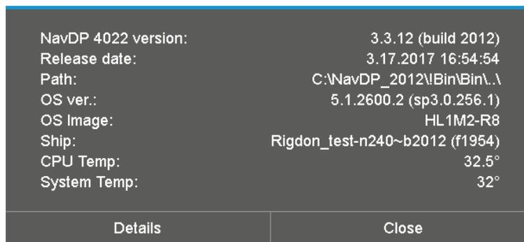
Figure 10.91: CPU and System Temperature in the “Info” Window
