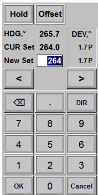
Figure 10.53: Input Heading Setpoint dialog
