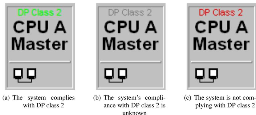
Figure 10.99: DP Class 2 Indication on the “Master CPU” Panel
