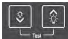
Figure 2.18: The Brightness Pushbuttons
