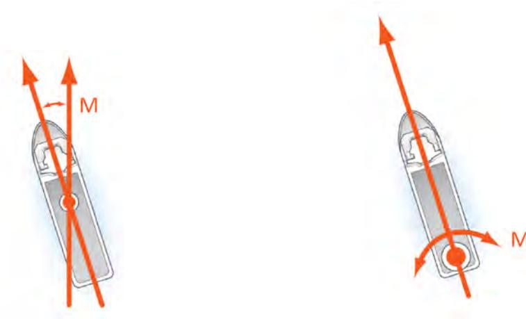
Figure 9.1: Manual Heading mode
