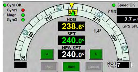
Figure 10.51: The Autopilot Heading Indicator
