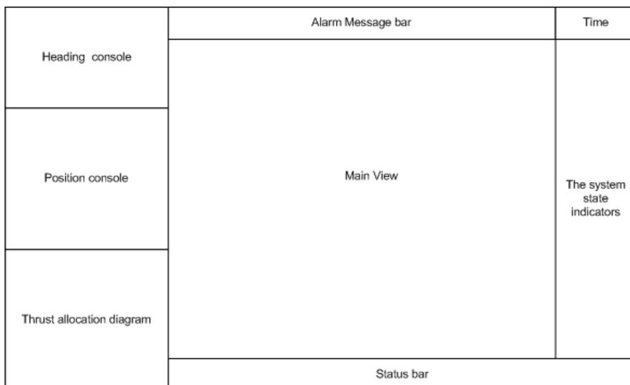
Figure 5.41: The Screen Operational Areas Layout
