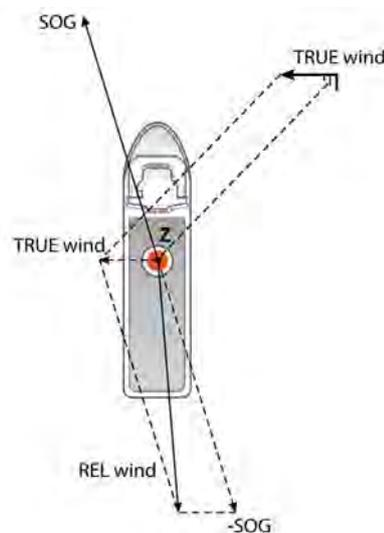
Figure D.1: True and relative (apparent) wind
