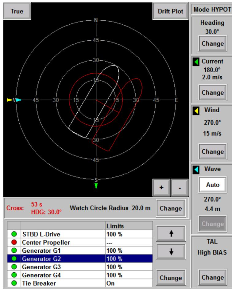
Figure 10.74: Drift Plot Window
