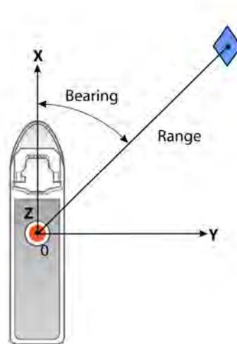
Figure 10.18: Single Target Following Mode: Coordinate Systems
