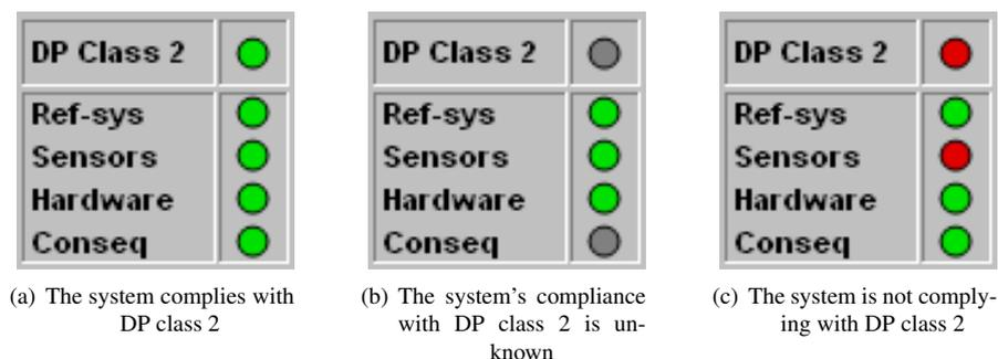
Figure 10.100: DP Class 2 Indication in the “System Monitor” Window
