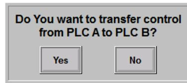
Figure 10.95: Example of the Dialog Box for Active PLC Change
