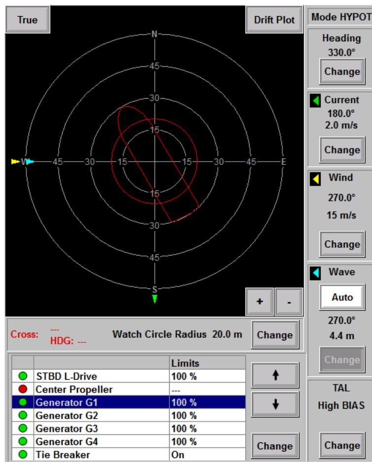
Figure 10.75: Drift Plot View without Vessel's Drift
