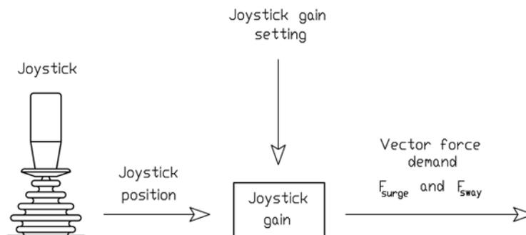
Figure 2.34: Joystick gain diagram
