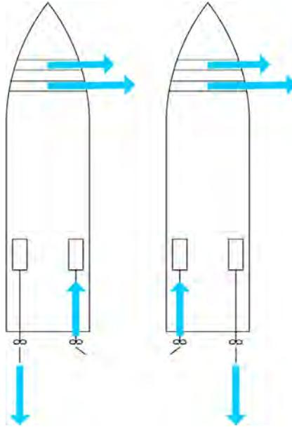
Figure 6.29: Thrust Allocation Modes: Starboard Ahead and Port Ahead
