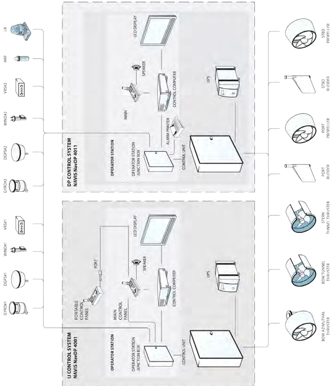
Figure 2.2: Typical NAVIS NavDP 4000 for DP-1 Class Ship Hardware Configuration
