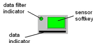
Figure 7.3: Sensor softkey with indicators
