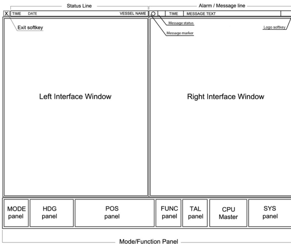
Figure 5.1: Operator Screen Layout
