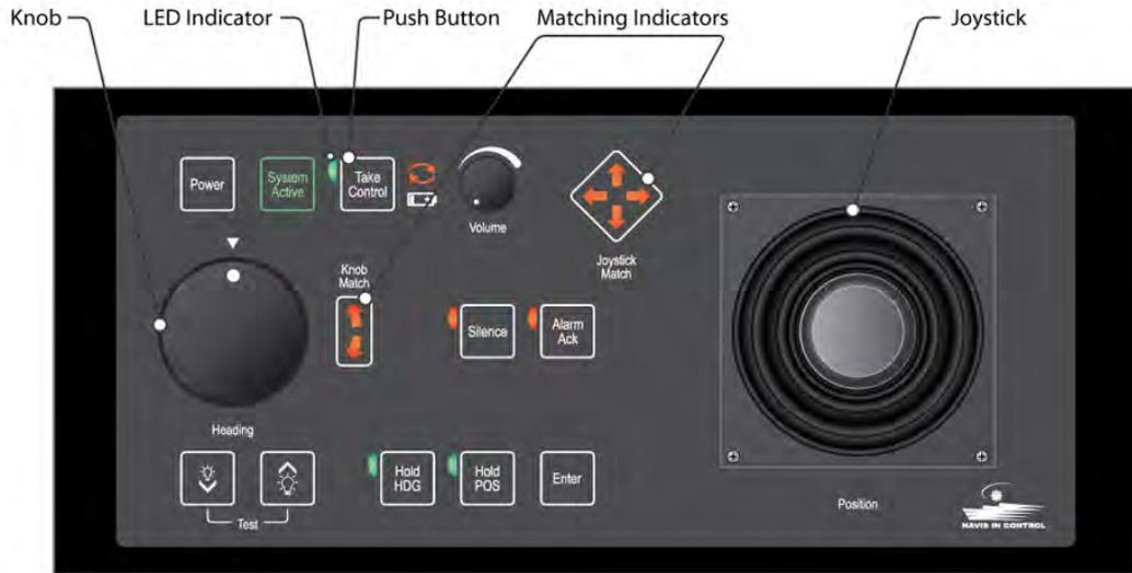
Figure 2.24: Control Panel Controls, Buttons and Indicators (MCP and PCP)
