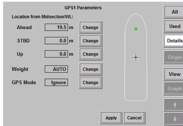
Figure 8.20: The GPS parameters window. Standard view
