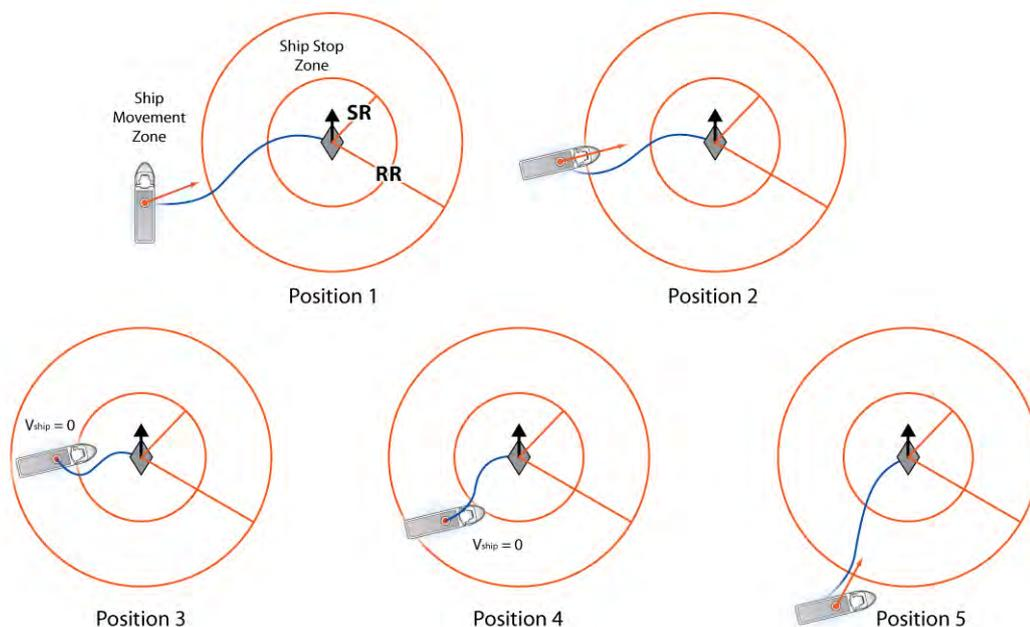
Figure 10.20: Reaction Radius
