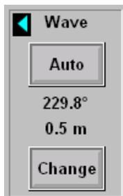
The values for wave direction and height set in the dialog box are displayed under the **Wave** text in the manual mode.
