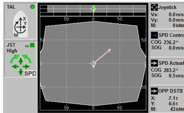
Figure 6.3: The required speed values in **Speed VECTOR** mode
