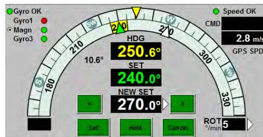
Figure 10.52: The Autopilot Heading Indicator. New heading input
