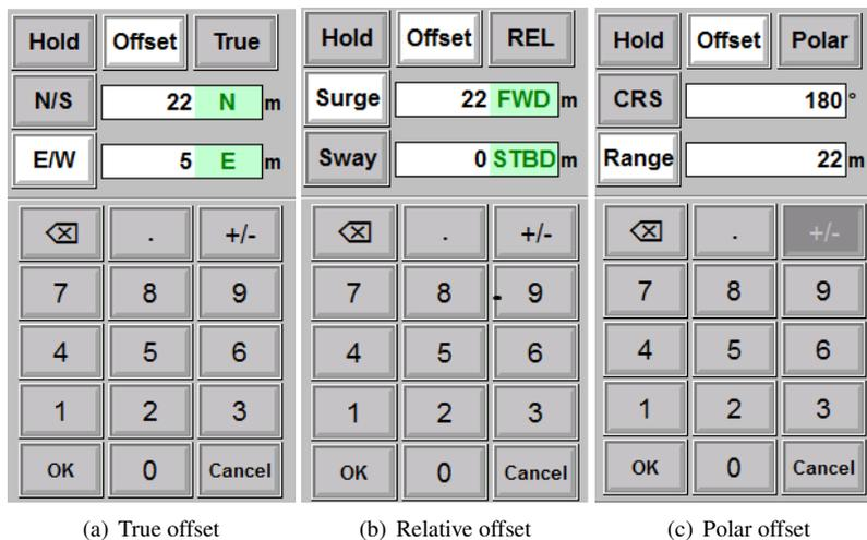
Figure 5.19: Input Position Offset dialog
