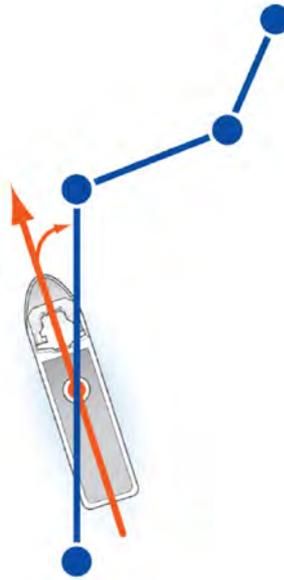
Figure 9.6: Low Speed Tracking
