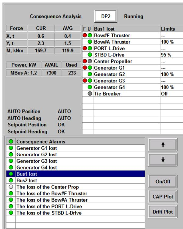
Figure 10.84: The Consequence Analysis Window Example
