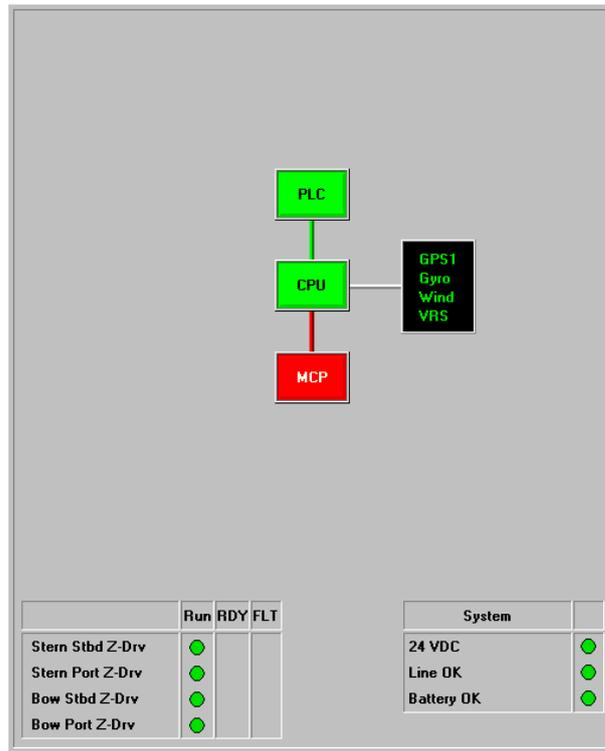
Figure 10.92: System Monitor Window Example — DP Class 0 System
