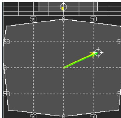
Figure 5.55: Thrust Ability Diagram (DP Mode)
