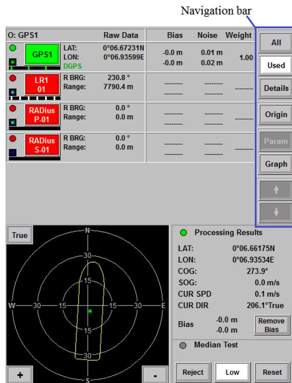
Figure 8.7: The position reference system window
