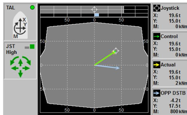
Figure 10.8: Thrust ability diagram. AWC function is OFF
