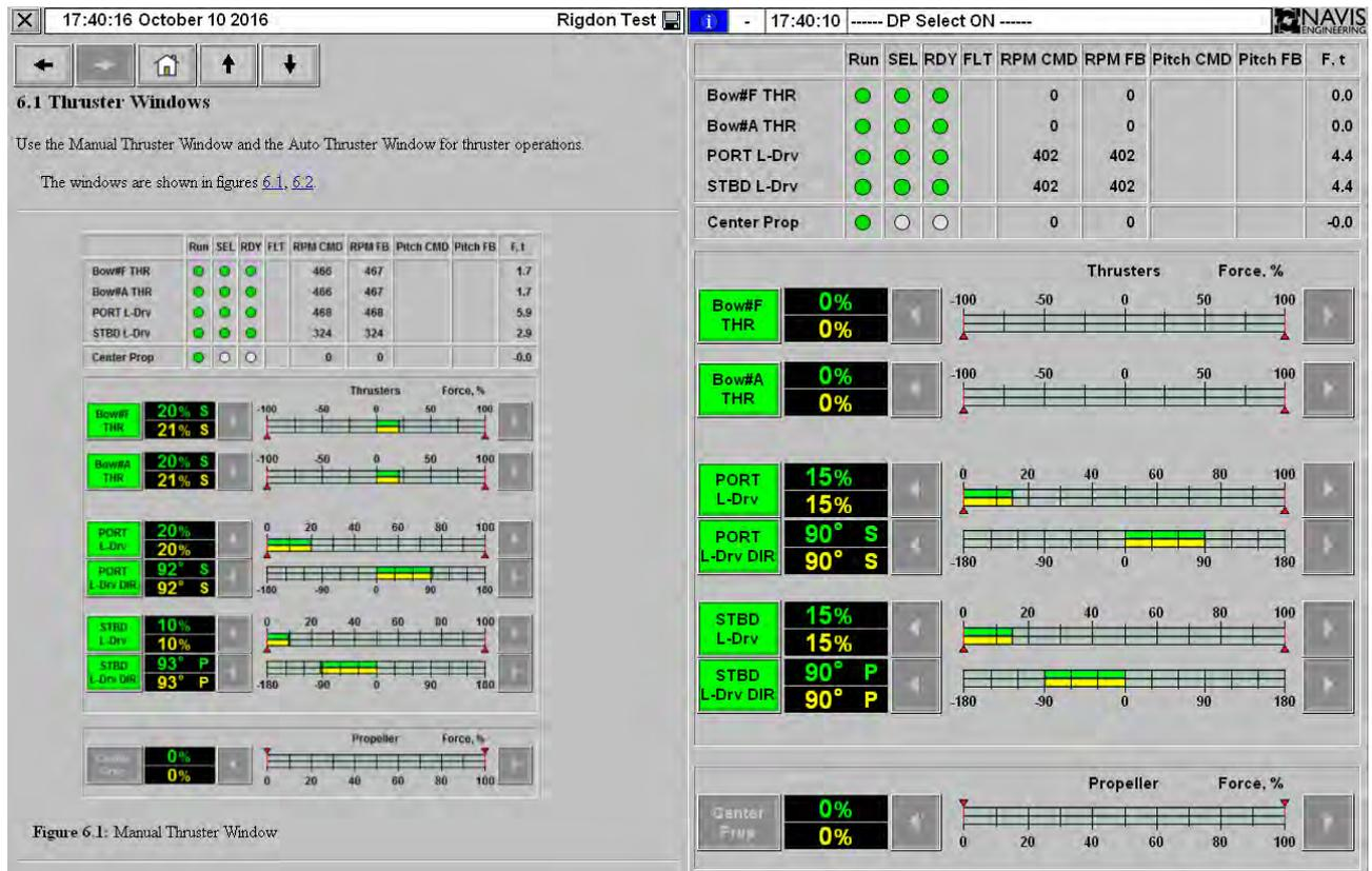
Figure 5.12: Help Window (Manual Thruster Section) — Manual Thruster Window
