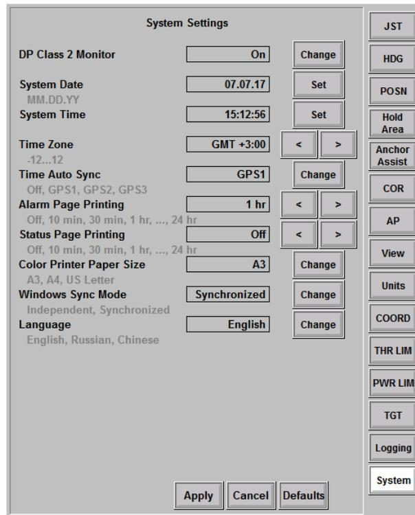
Figure 5.37: The setting mode on the System tab
