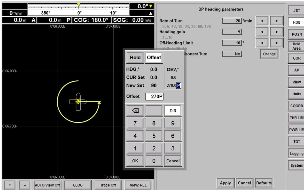
Figure 5.24: The turn track in case Always Use Shortest Turn=No
