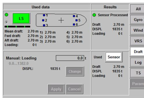
Figure 7.19: Draft sensor details
