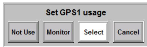
Figure 8.11: Dialog Box for the sensor in case it is Selected or cannot be used as target
