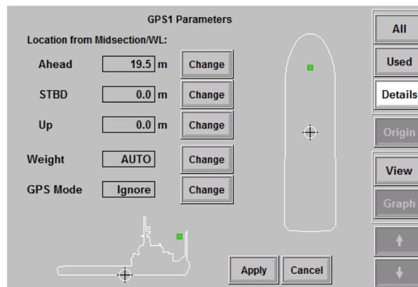
Figure 8.21: GPS parameters with the side view
