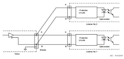
Figure 7: IEC 61162-1 Circuits
