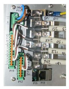
Figure 10: Serial pin connections
