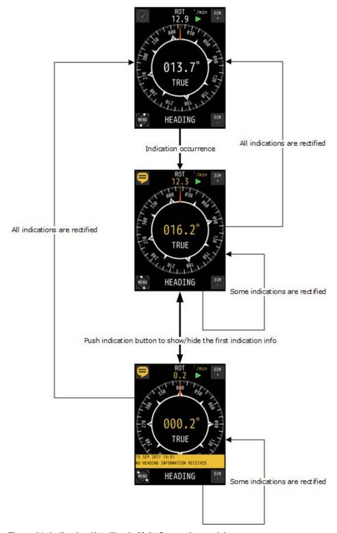
Figure 21: Indication Handling in Main Screen (example)
