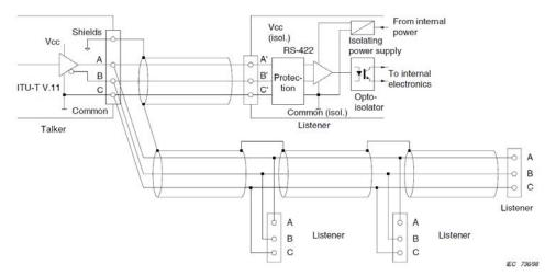
Figure 8: IEC 61162-2 Circuits
