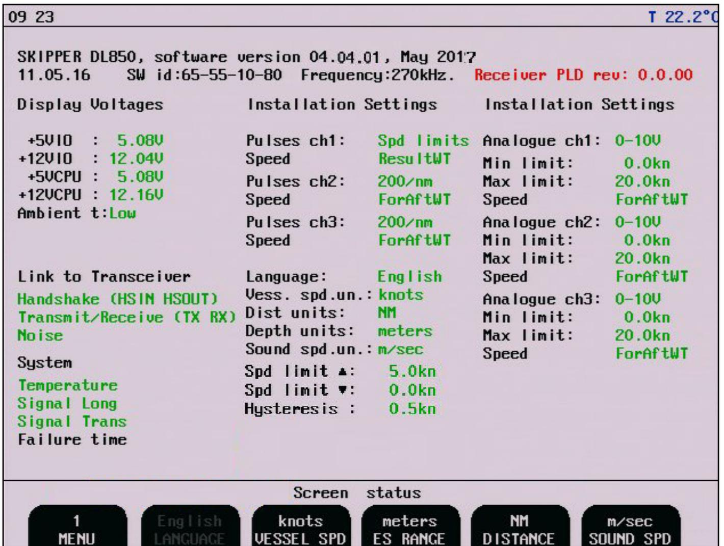
**Important note:** If, after power-up, on screen status, you see the following message “Receiver PLD rev: 0.0.00” in the upper right corner, this is an indication of old PLD in the transceiver unit. The unit will work, but is not optimized. Replace PLD with correct version, (1.0.00) or contact your local supplier for more information.
