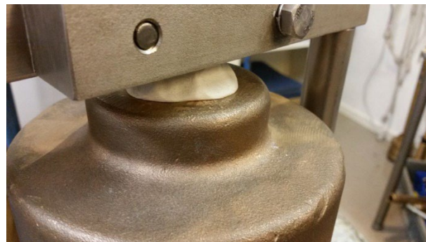
Figure 3. Non-hardening soft putty applied around the connecting tube on top of the valve cover
