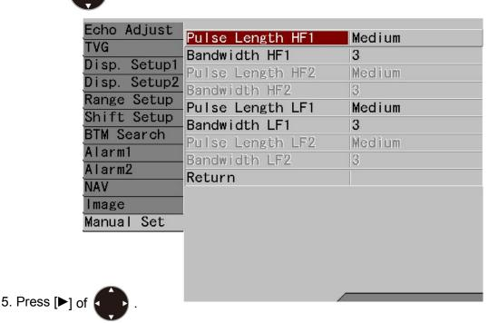
6. [Pulse Length HF1] of the menu is displayed. Move the cursor with [▲] or [▼] keys of ♠, and select one of [Short], [Medium] or [Long].
