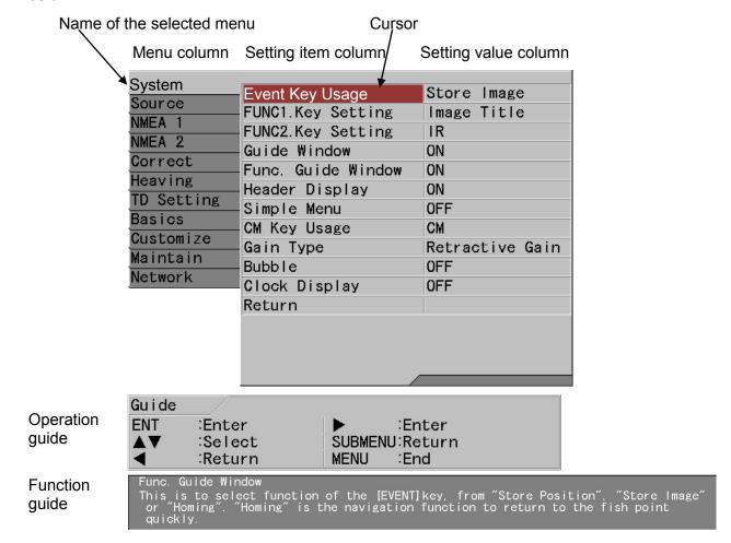
The operation guide is displayed when [SUBMENU], [System] and [Guide Window] are all on. (See the Instruction Manual [Advanced] "5.2.1 Display/No display of Guide Window") The function guide is displayed when [SUBMENU], [System] and [Func. Guide Window] are all on. (See the Instruction Manual [Advanced] "5.2.2 Display/No display of Func. Guide Window")
