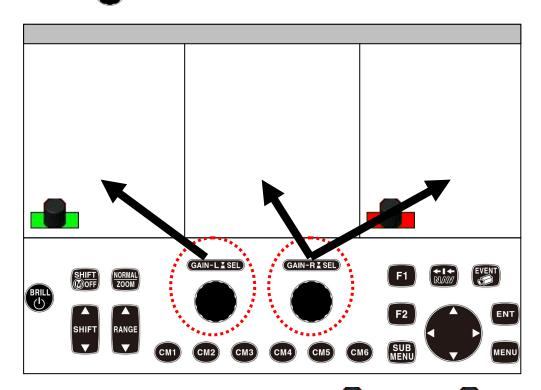
The gain can be adjusted of the screens on which knob icon] on the lower left of screen are displayed. \_\_\_\_\_
