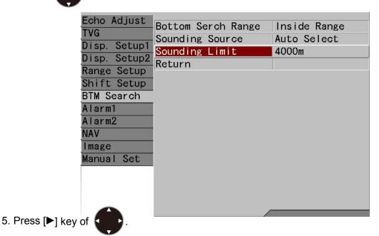
6. The menu [Sounding Limit] is displayed. Adjust the depth by increasing/decreasing the value with [▲] or [▼] keys of .
