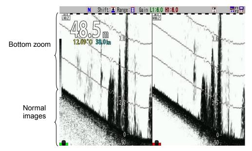
Mixed images above bottom in a specified zoom range are displayed onto the normal image.
