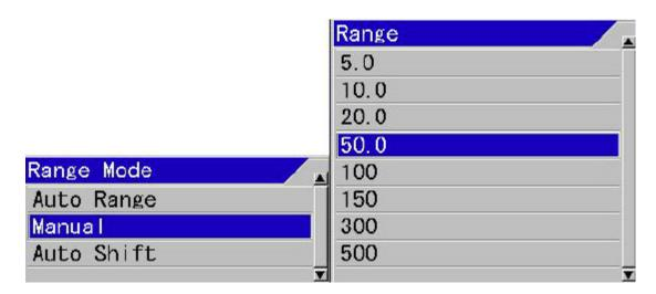
3. Press [ENT] key ENT . Then, [Manual] is set and the header showing the Range Mode disappears
