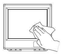
For cleaning the chassis, do not use solvent such as thinner or alcohol. Painting on the surface and characters at the Operation unit may be dissolved. After wiping with soft and clean cloth dipped with diluted neutral detergent, wipe away with dry soft and clean cloth.
