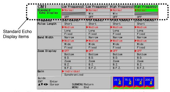
When [Normal] is selected, normal images are displayed on high frequency 1 screen. When [OFF] is selected, high frequency 1 screen is not displayed.
