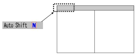
Caution: During the operation of auto shift, [Shift] key is disabled. In addition, the shift operation is set to [All Screen Same], and the [Scr. Individual] range and the [Scr. Individual] shift are not available either.
