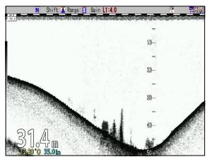
Image after rejection of interference
