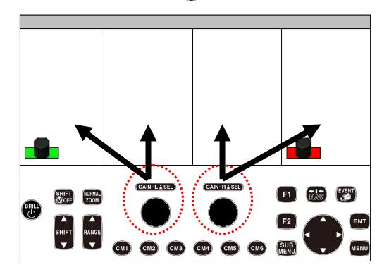
The gain can be adjusted of the screen in which [Gain knob icon] of (red) or (green) is shown at the lower left of screen.
