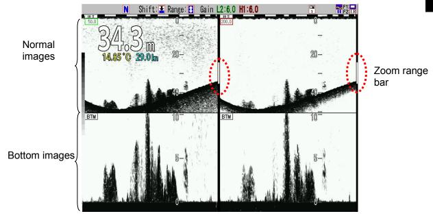
Sea bottom is fixed at 10% bottom of the screen, and the image above is displayed in the specified zoom range. As the image on sea bottom is magnified, this is an effective zooming mode to identify fish schools, etc. near the bottom.
