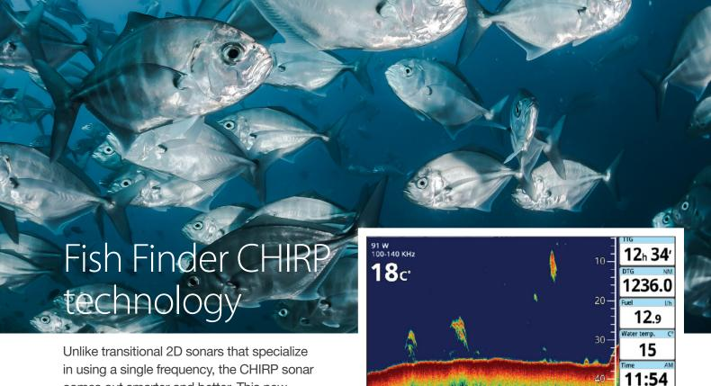
in using a single frequency, the CHIRP sonar comes out smarter and better. This new technology eliminates surface clutter and water column noise, for Hi-Fi visibility.
