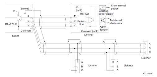
Figure 10: IEC 61162-2 Circuits
