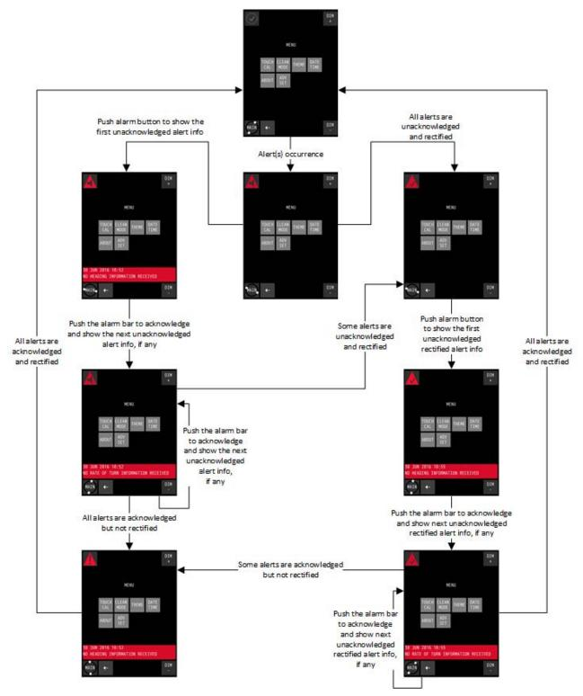
Figure 21: Alert handling in menu (example)
