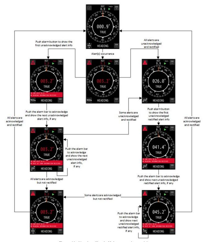
Figure 20: Alert handling in Main screen (example)
