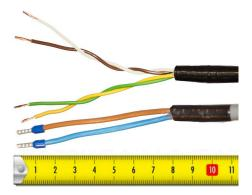
Figure 7: Cable Preparation Receiving Cable Sides
