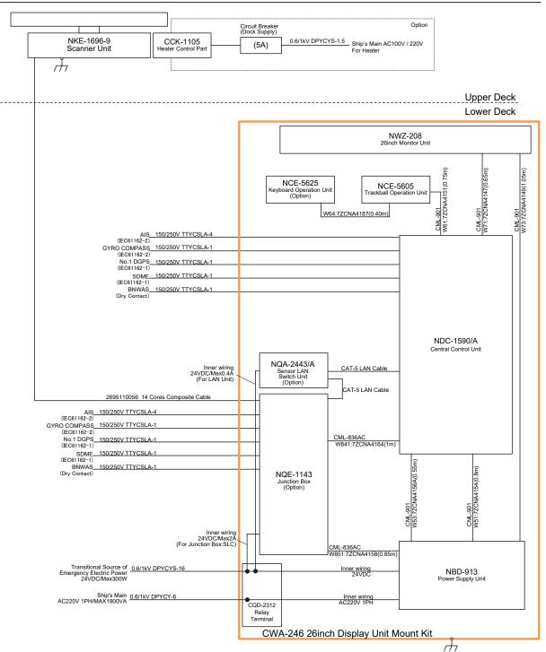
NOTE: ELIMINATING THE INTERFERENCE ON FREQUENCIES USED FOR MARINE COMMUNICATIONS AND NAVIGATION DUE TO OPERATION OF THE RADAR, ALL CABLES OF THE RADAR ARE TO BE RUN AWAY FROM THE CABLES OF RADIO EQUIPMENT.
