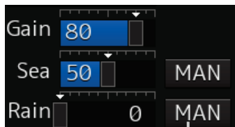
AUTO Rain/Snow Clutter Suppression button
