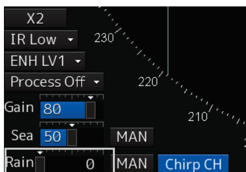
[Rain] (rain/snow clutter adjustment) slider
