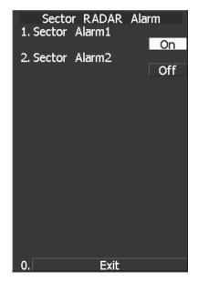
**Note:** When the automatic acquisition / activation zone key allocation is set, pressing the **[AZ]** key will simultaneously turn on or off the radar alarm in the automatic acquisition / activation zone.
