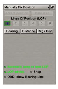
The OBD continuously transmits bearing information to the MFD. This allows the ECDIS task screen to provide a real-time display of an Optical Bearing Line – showing what the OBD operator is looking/pointing at.
