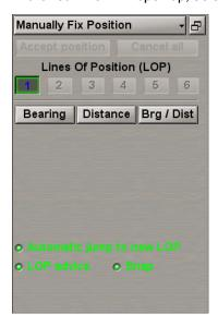
The **Manually Fix Position** display is intended for constructing the ship line of position (LOP) by measuring bearing and/or range to one or more visible objects whose coordinates are known in advance (or the object can be uniquely identified on the chart).
