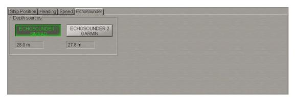
The **Echosounder** page is designed for selecting a depth source. The **Echosounder** page shows all the connected depth sensors.
