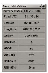
The **Primary Status** page is used for presenting the following data from the EPFS used as the primary positioning system:
