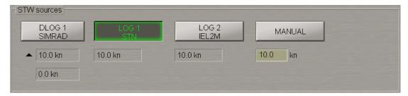
The **STW** sources group is designed for selecting a source of speed through the water. The group shows all the connected speed-through-water sensors.
