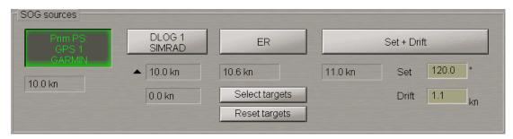
The **SOG** sources group is designed for selecting a source of speed over ground. The group shows all the connected speed-over-ground sensors.
