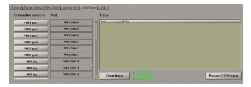
This page is intended for displaying and recording of the IEC 61162-1, 61993-2, and proprietary formats and similar text messages/sentences provided to the MFD from the external sensors and displaying of the sentences transmitted by the MFD to the external devices.
