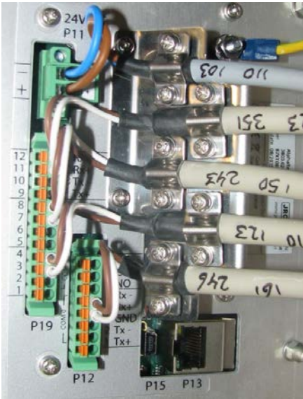
Figure 14: Serial pin connections
