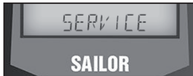
Figur 4 - Once connection between the Service Tool and the radio has been established thus activating the radio in service mode, this will be indicated in the radio display by reading “SERVICE”.
