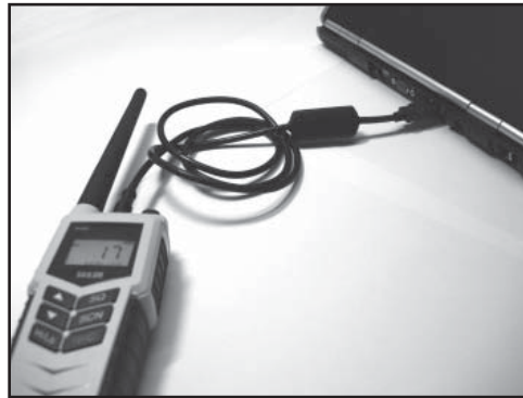
Figure 1 - Simple connection between service PC and radio.
