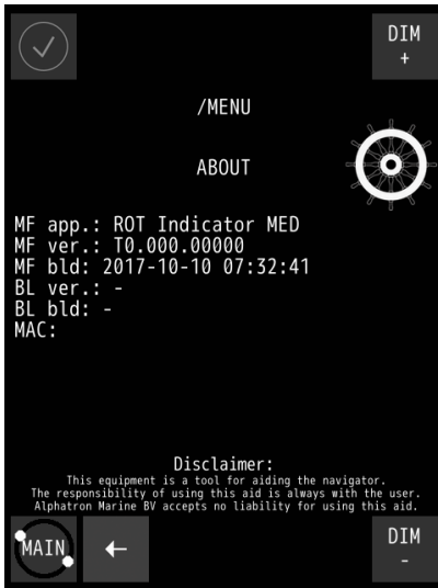
Figure 28: About the ROT Indicator
